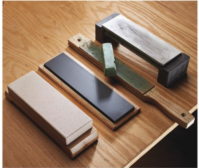
Polish. Here's where things get crazy; polishing media goes to great heights on the grit scale. Pictured front to back are a #16,000-grit Japanese waterstone, a hard Arkansas oilstone, green stropping compound and an #8,000-grit no-soak waterstone (that a student gouged).
