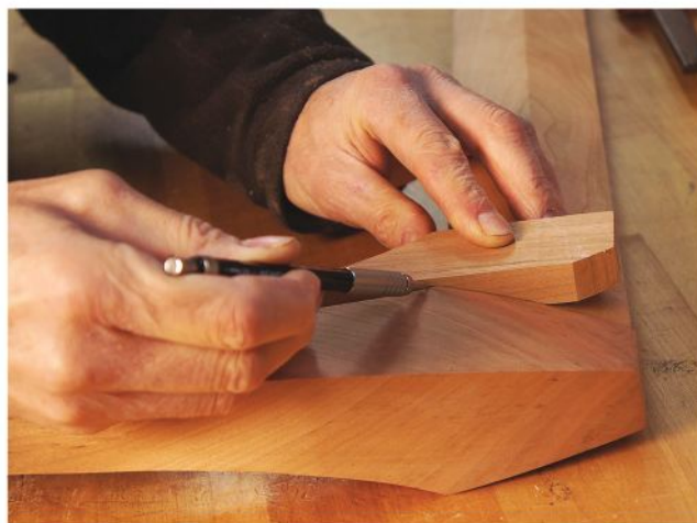
Direct line. With the knee block in position, mark the curved edge where the block meets the leg.
