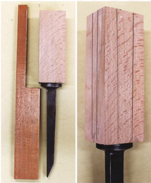
Handle gauge. This shop-made layout jig keeps my lines centered off the chisel's shaft.
