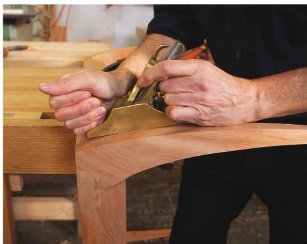
Uphill battle. Pay attention to grain direction as you work on the curved surface of the leg and knee block.
