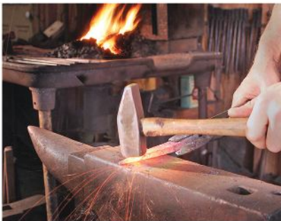
Smith. Peter Ross shapes the "burner" tang at his anvil (if you're smithless, you can shape your burner by sawing, grinding and filing).
