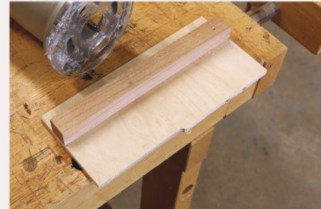
Dialed-in location. Running the router up the assembled jig cuts the jig exactly where the edge of the router bit does its work.
