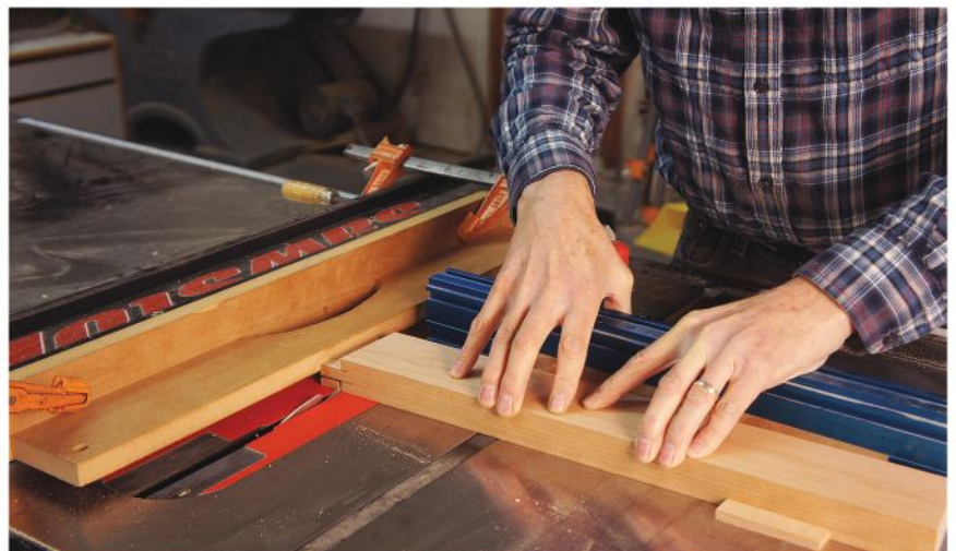
Fence & wedge. The auxiliary fence prevents offcuts from being trapped between the blade and fence. The wedge is used to quickly set the proper angle.
