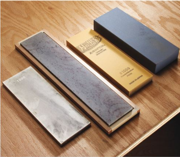
Hone. From front to back are pictured a #1,000-grit diamond stone, a soft Arkansas oilstone, a #1,000-grit no-soak waterstone and a #1,000-grit Japanese waterstone.
