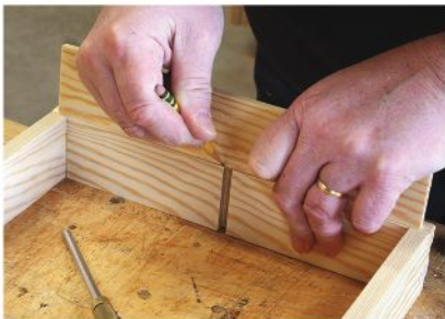
Two procedures. Set the parts – short dividers at the ends and longer dividers at the sides – in position on the box or tray as you transfer the layout.
