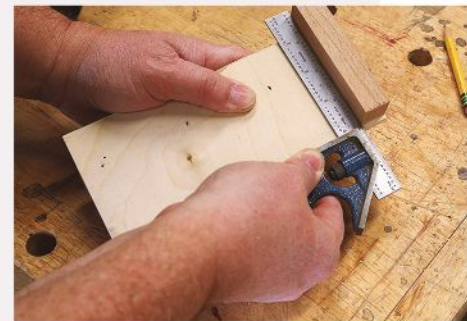
Get it square. The usefulness of this jig depends on the T-square piece being set at a perfect 90° to the base.
