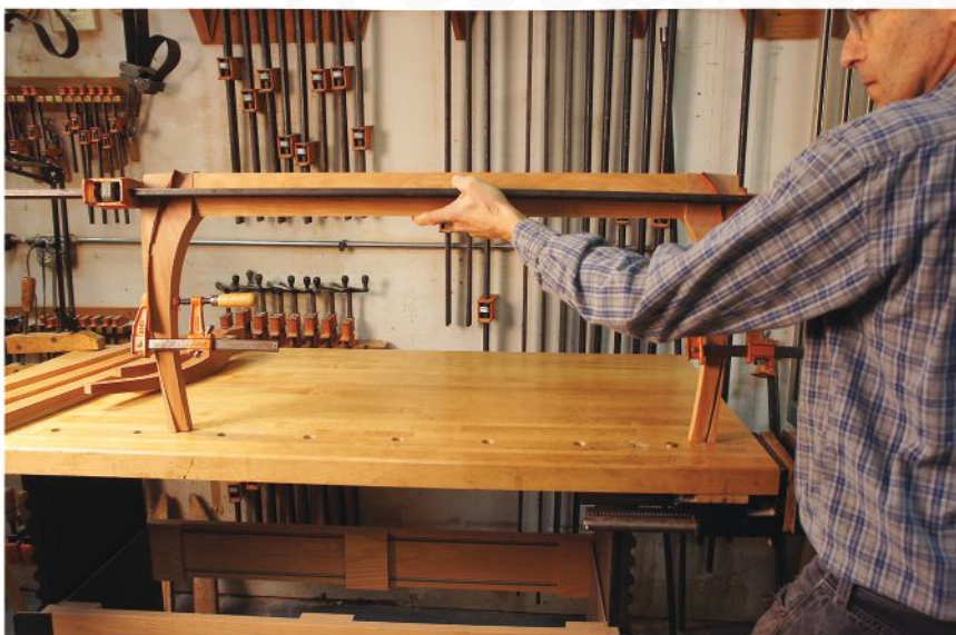
Offcuts again. The waste from cutting the legs provides a flat surface that keeps the clamps from slipping as they are tightened.
