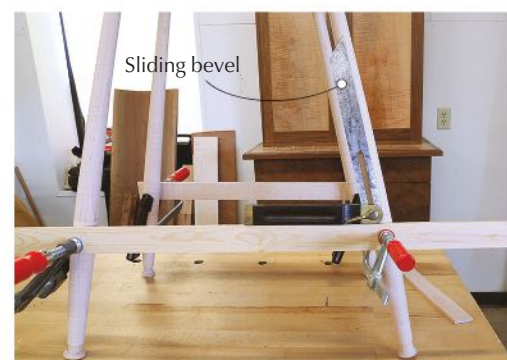
Angle it. Clamp scraps to the dry-assembled base and set a bevel to the centerline of the leg. This will be the angle at which you will drill the holes for the stretchers.
