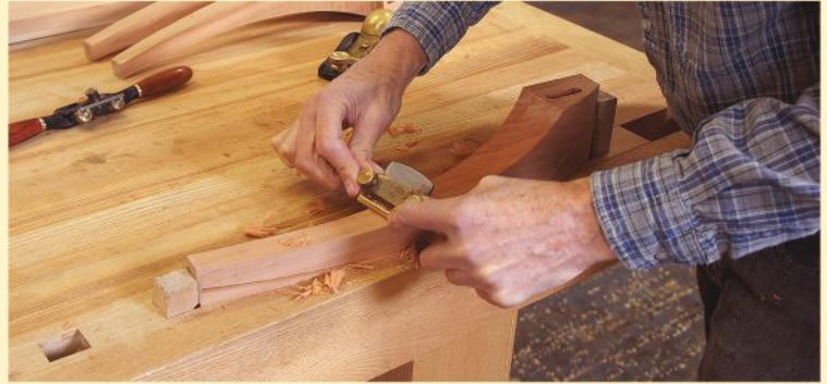
Save the scrap. The waste from cutting the legs is used for support while cleaning up the concave inner surface.
