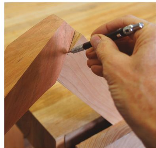
Right angle. The end of the apron falls in the middle of the curve. Fit the apron in the leg and mark to bevel the top of the apron.
