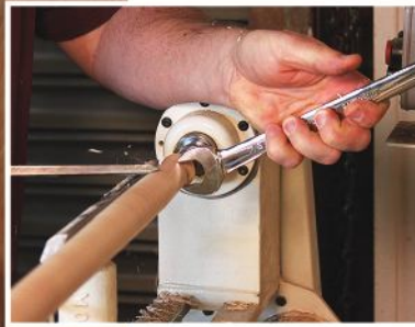
Wrench it up. A fairly simple turning trick to get consistent sizes is to use a wrench as a caliper.
