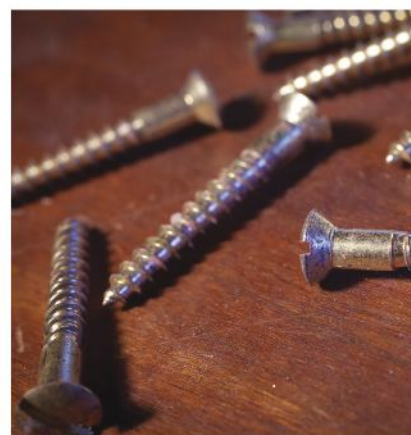
Screw details. The most important detail here is the diameter of the screw's head right where the slot bottoms out. That will be the diameter of your finished "rivet" and is the maximum diameter of your countersink. With these screws, that diameter is .325".
