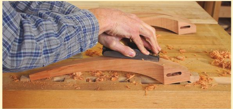
Low dogs. The outer convex curves are easier to hold, but keep the dogs out of the path of the block plane.
