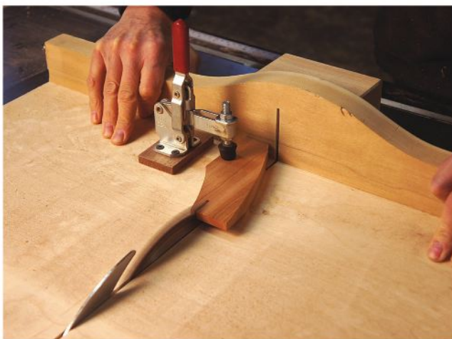
Straighten out. The first step in making the transition blocks is to create a straight edge that butts against the flat surface of the leg.
