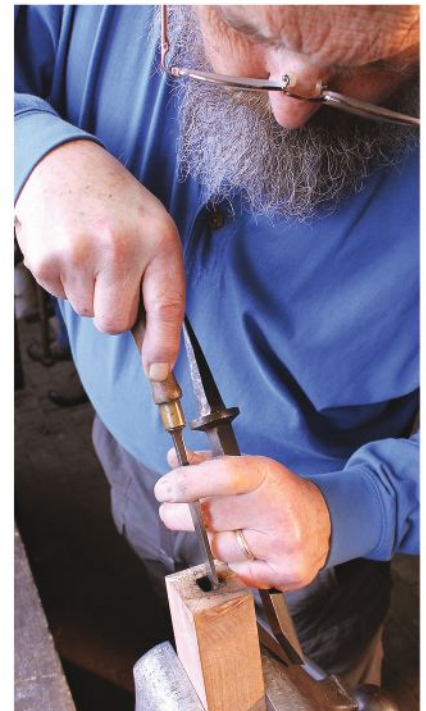
And test. With the hole burned out, I test the fit of the chisel tang.
