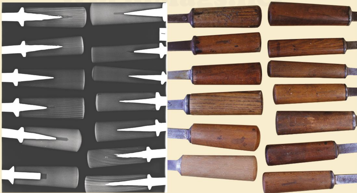
Inside & out. An X-ray reveals the tangs inside oval-bolstered mortise chisels.
