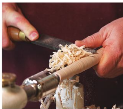
Skewed turning. Work from the largest diameter towards the smaller diameters when turning. This is particularly important when turning the slender tenons on the stretchers.
