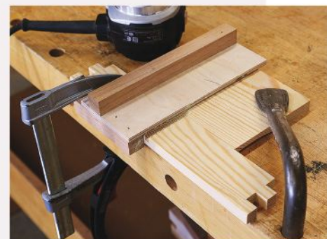
In action. Here you see the dado jig in action – you also see a backer that eliminates any blow-out as you cut the tray parts.
