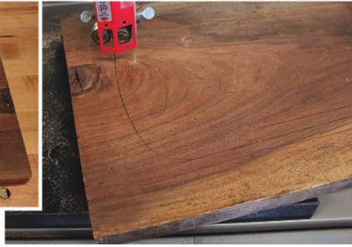
Rough cut. Careful placement of the pattern allows the seat to be defect-free. The band saw makes short work of roughing out the seat blank.
