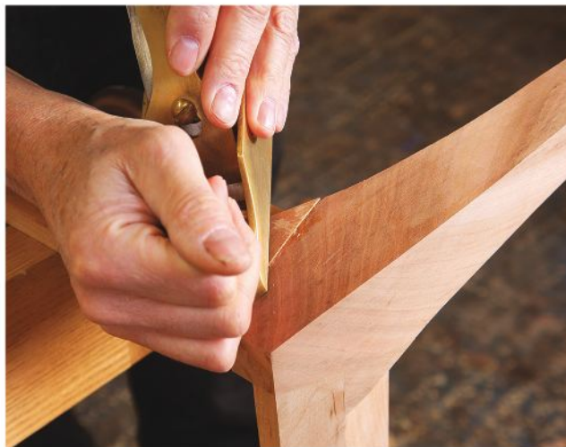
Make it match. Cut the block a bit thicker than the leg, then plane it down to blend the two pieces.
