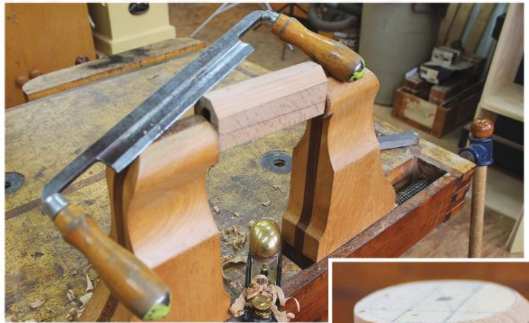
Shaping setup. My clamp for this sort of work resembles a lathe's headstock and tailstock. It holds the work securely as I shape the oval handle with a drawknife, block plane and spokeshave.
