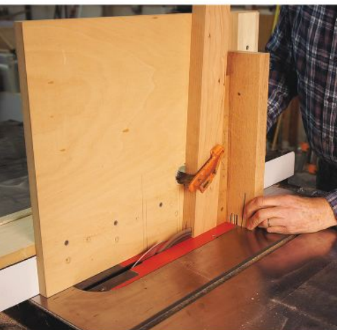
Wise wedge. A simple wedge behind the angled aprons allows the cheek cuts to be made with this tenon jig.
