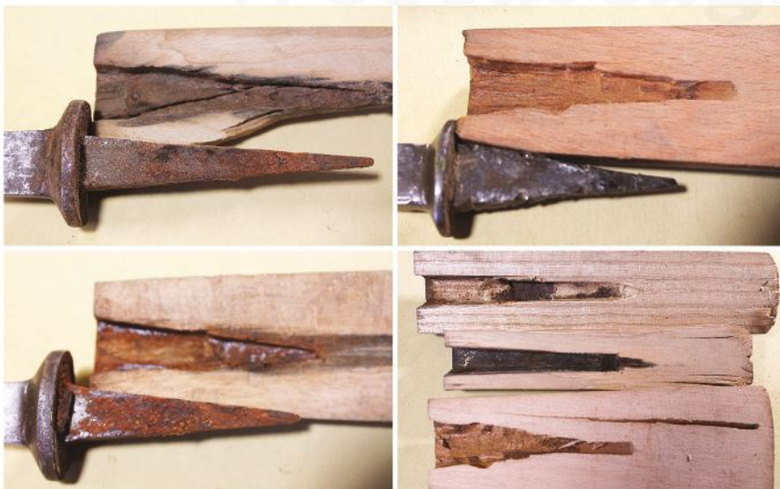
Scorched remains. The black coloring inside these broken handles provides evidence that the tangs were burned in to the wood.
