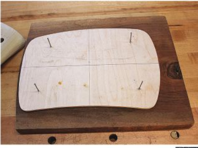
Pattern seating. Choosing your figure and grain direction is crucial for a sturdy stool. The nails in the pattern help locate the center of the leg holes.
