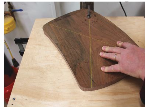
Angle drill. Using a shop-made jig, the leg holes are easily bored at the selected angle.
