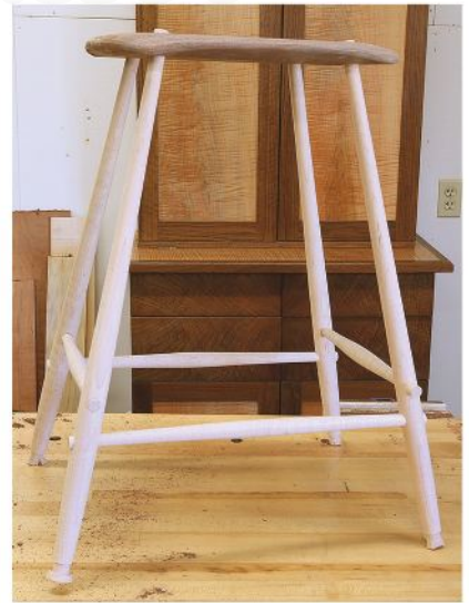
Dry-fit. Rough assemble the stool and trim the tenons close so the wedge placement can be marked.
