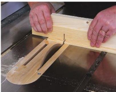
In plain view. Drawing a bead on where to position your egg-crate cuts is straightforward because you can easily see the slot cut in the carrier.
