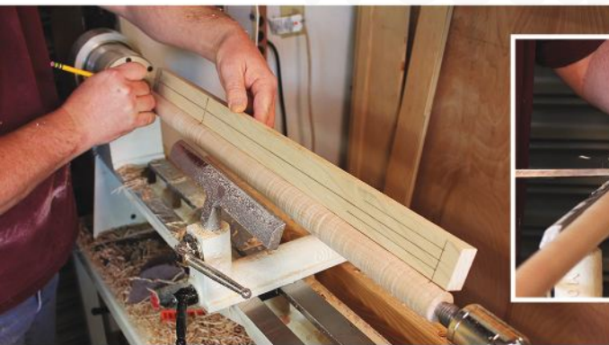
Layout sticks in action. After turning the leg blank to a 1¼"-diameter cylinder, use the layout stick to plot the top and bottom, and the middle of the swelled part of the leg.
