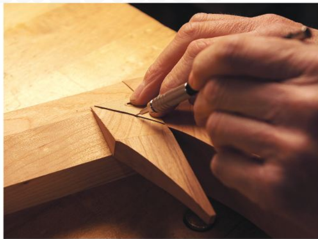
Follow along. The curve of the leg continues into the transition block. A cardboard pattern ensures consistency.
