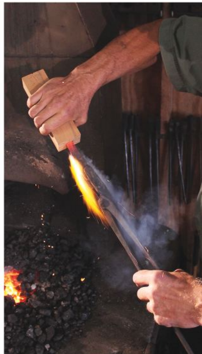
Burn. Peter inserts the heated burner into the pilot hole.
