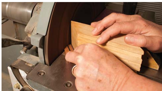
Perfect miter. In lieu of a shooting board, it's easy to sand the inlay miters using a 45°-guide block at a disc sander.
