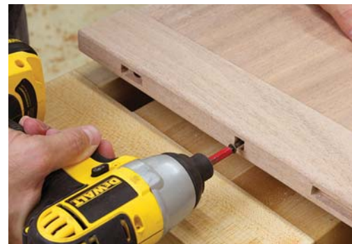
Undercover. Ebony plugs will cover the screw heads after the breadboard ends are attached.
