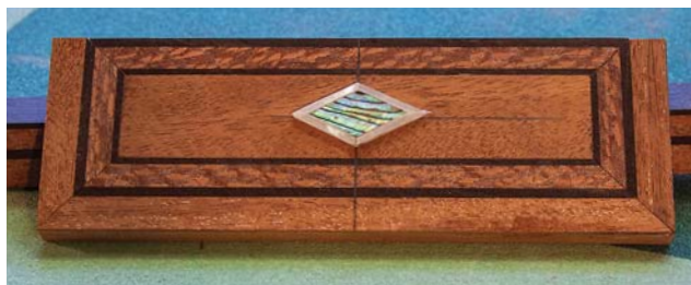
Shell diamonds. After gluing on the wooden inlays, center and inlay the paua abalone and mother-of-pearl diamonds.
