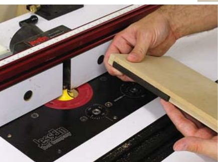
Hands back. This simple made-from-scrap jig holds the ebony bar so the profile can be safely routed.
