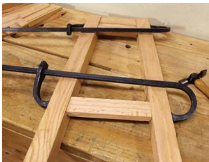
Benchless holdfast. The mechanics of these iron bar clamps are similar to those of a holdfast.
