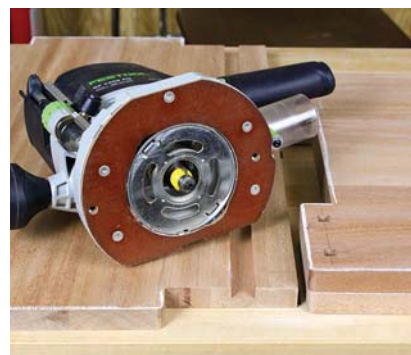
This, not that. Mark the edges to be rounded over with chalk to help prevent shaping the wrong edges.
