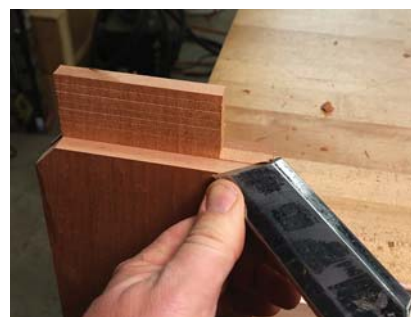
Paring. Use a chisel to clean up the shoulder after you've cut the haunch.
