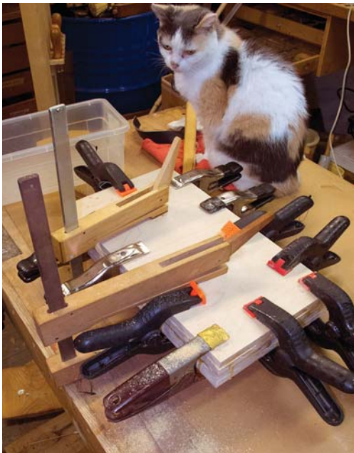
Quad-layer spacers. Blocks of four layers of Baltic birch plywood are glued with hot hide glue and standard shop clamps. All of the wood components in this project are Baltic birch plywood.
