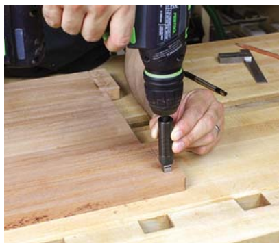
Two steps. Mortises for the ebony plugs are created by punching a square hole, then removing the waste with a drill.
