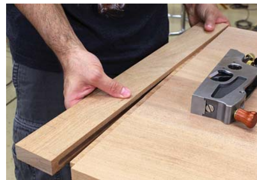
On the end. The groove in the breadboard end fits over the tongue of the top panel. Screws in oversized holes hold the two pieces together.
