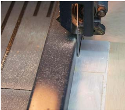
Save some money. Mother-of-pearl and paua abalone strips cost significantly more when pre-made. It's a snap to cut them on the band saw.
