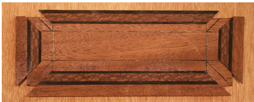
Fit wood inlay. On the box's front, back and side panels, draw the locations for the wood inlay pieces and miters, then cut each piece to fit.
