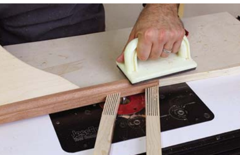
Double duty. The curved template is used as a router fence that supports the arched handle while the cove profile is routed.
