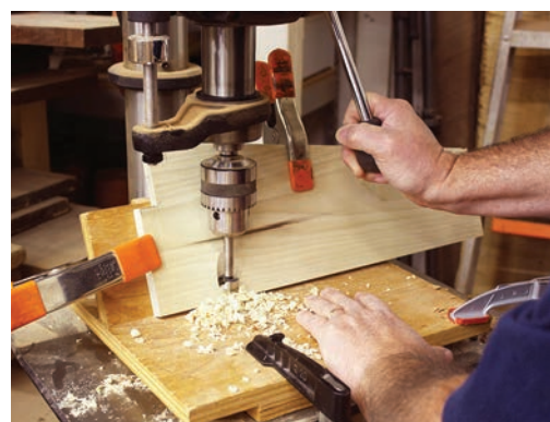
Laid back. The key to good pocket-screw holes using a press is to tilt the workpiece at 22 \frac{1}{2} ° as you drill.
