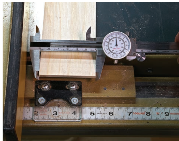
On the mark. A sacrificial board attached to the miter gauge makes it easy to align marks to the path of the blade.
