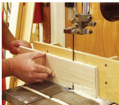
Tapered parts. The band saw is the best way to taper drawer parts. Make sure you leave material to plane the surfaces smooth and still hit the appropriate thicknesses.
