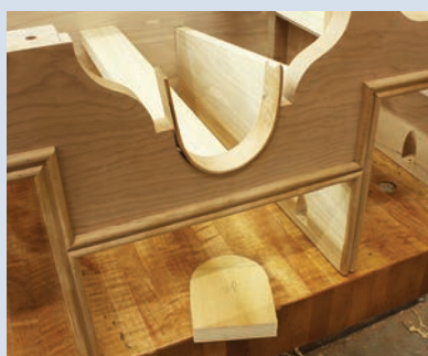
Works great. I found heat bending was excellent for the larger radius bends, and for the round center section. Do use a form.
