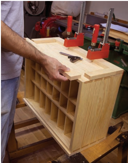
Piece by piece. The battens form the rails and stiles that frame the exterior walls of the crate. As on the original, they are simply nailed and glued to the carcass – there's no joinery between the rails and stiles. So this is fast work.
