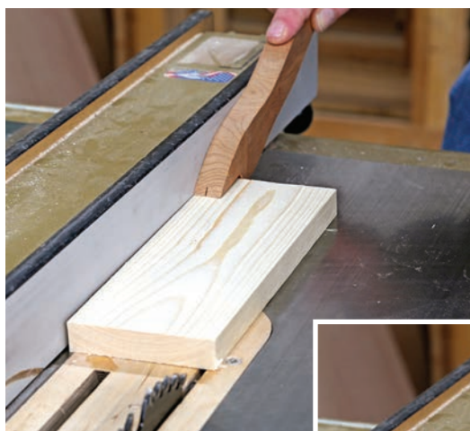
No help. Pushing stock from near the fence tends to move the opposite corner into the blade, inviting kickback.
