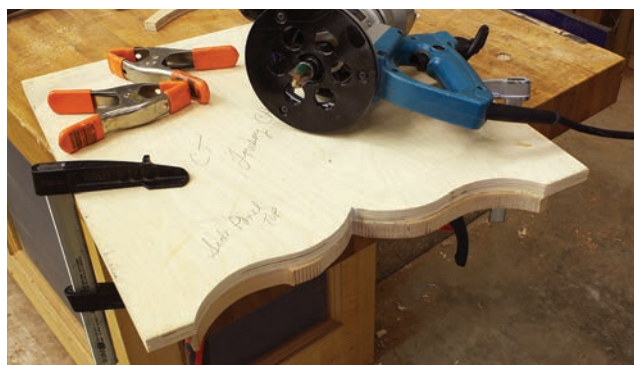
Fast & accurate. Pattern work made with a router setup is quick and easily repeated when needed.
