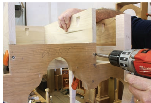
Hidden stability. A couple of well-placed screws – that will be covered by double-arch mouldings – hold the dividers tight to the apron.
