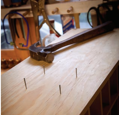
Affix the dividers. With the lines drawn on the carcass sides, drive in the cut headless brads and set them 1/16" below the surface.
