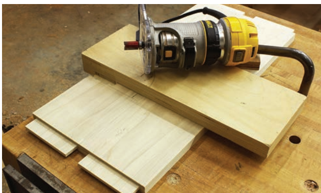
Square-platform jig. I find this setup to be one of the most repeated operation in my shop. Here I'm using a \frac{5}{8} " pattern bit.
