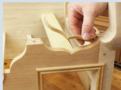
Look ma, no bends. It's possible to produce shaped cock beading that perfectly fits the cutout. The secret is pattern work.
