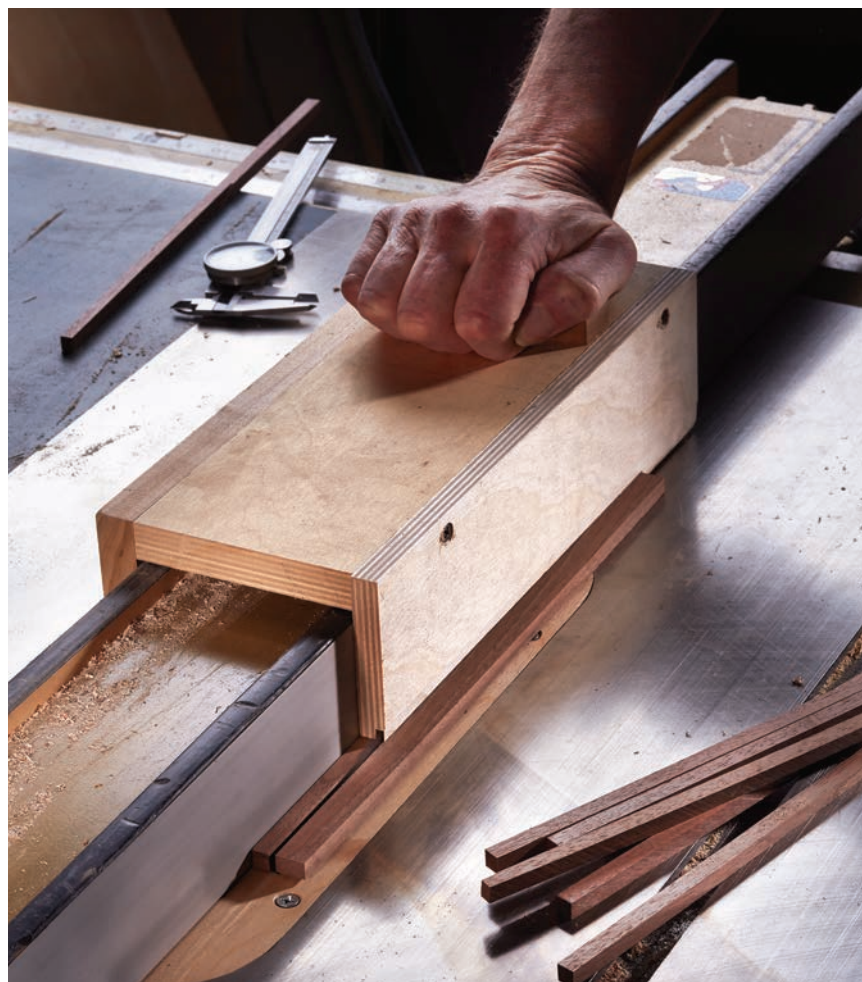
Think ahead. Small pieces (and large ones) can be cut on the table saw safely and accurately.
