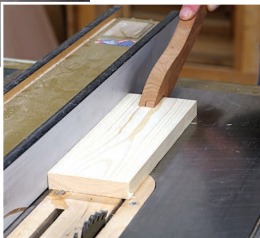
Into the fence. Pushing from near the center of the board increases leverage and keeps the leading edge of the material tight to the fence.
