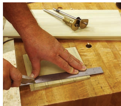
Forget a marking gauge. An easy technique to lay out the top and bottom thicknesses is to strike a line with a sharp knife registered against a straightedge.
