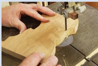
Test your skills. Cut close to the line, but don't touch it; excess material can be sanded away, but nicks mean you have to make another piece.
