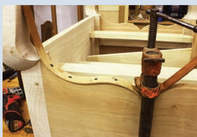
Old school. One technique used to form-bend the cock beading is to apply high heat to a soaked piece of moulding. The act of steaming the piece allows it to bend into shape.
