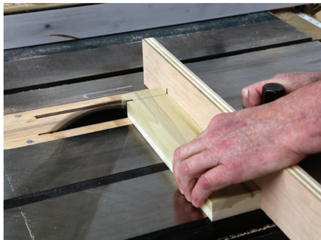
On the mark. A sacrificial board attached to the miter gauge makes it easy to align marks to the path of the blade.
