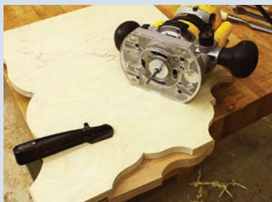
Synergistic. The correct combination of router bit and bushing produces a perfectly thickened piece for cock beading.
