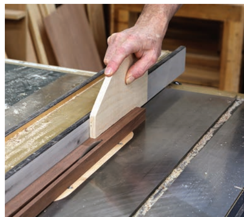
Down and forward. This type of push stick holds the work down to the table as well as pushing it into the blade.
