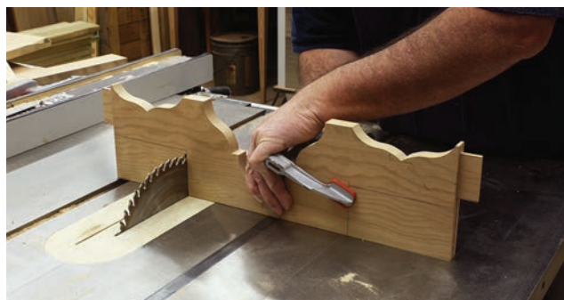
Choose your tool. The depth of cut to create the drawer opening can be reached at the table saw, but this operation could just as easily be completed using a handsaw.
