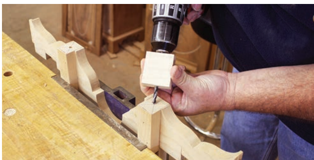
Simple jig. Holes for the drop finials have to be true; one easy technique is to use a drill press to drill a scrap to use as a guide for your power drill. Hold the scrap flat and tight to the apron as you work.
