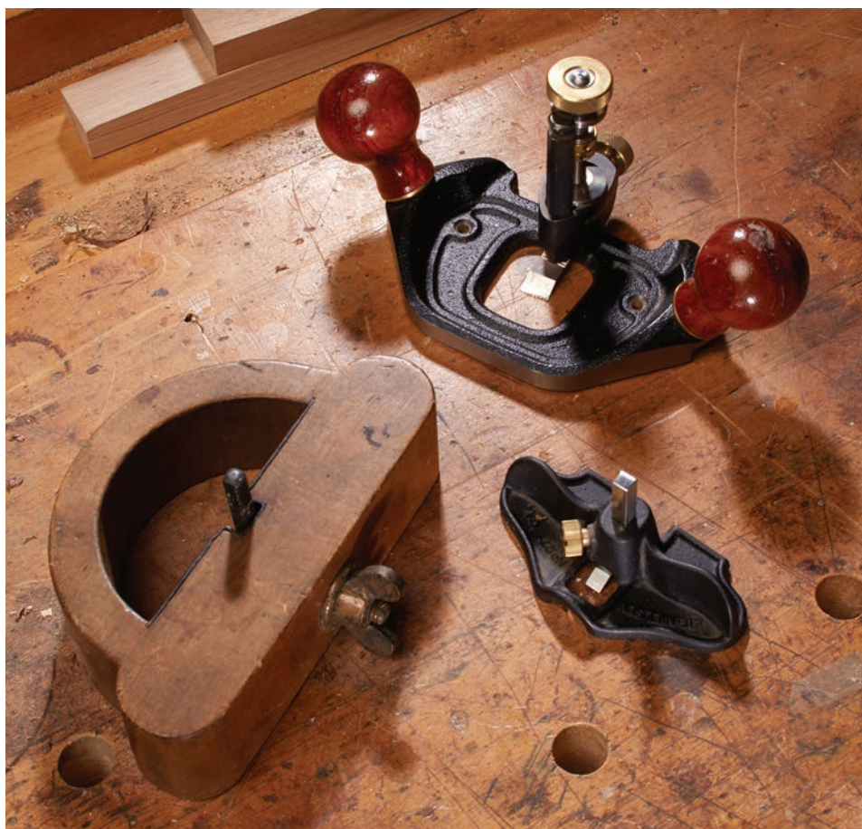
Large, small & shop-made. The large router plane at the top is a “vintage” Veritas (newer models have a more robust depth-stop mechanism); the small open-throat router plane is from Lie-Nielsen. The wooden D router plane was made by my grandfather.
