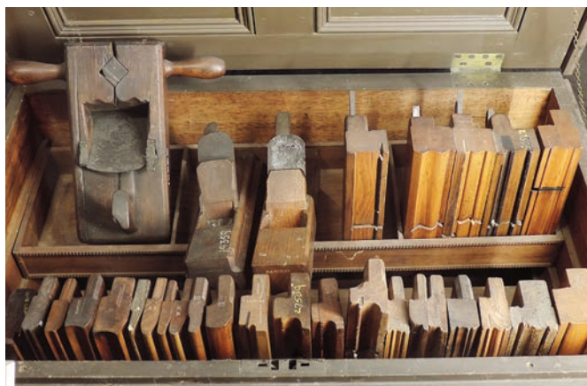
Moulding time This is just one of the tool chests in the woodshop at the museum; this one is filled with hollows and rounds, as well as complex moulding planes.
