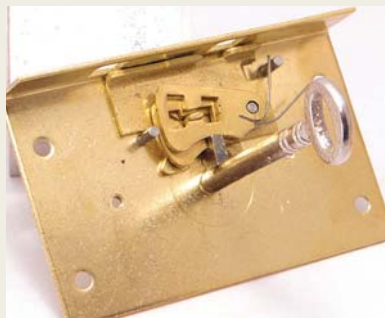
Lifted lever. At mid-turn, the key has engaged the levers and begins to clear the path to a fully unlocked position.
