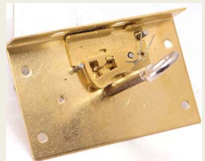
Mission completed. The main lever has slid to the unlocked position. The spring pushes the levers down to hold the lock open.
