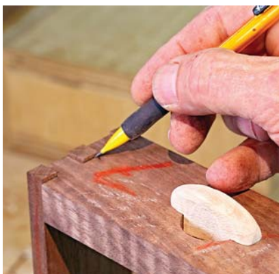
Make the target. The face of the drawer front is marked directly on the fingers of the drawer side in the dry-assembled drawer.
