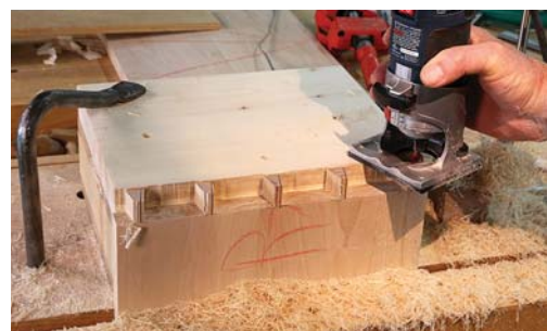
Rapid removal. A trim router with a straight bit makes quick work of clearing waste between the pins, and it leaves a flat baseline.
