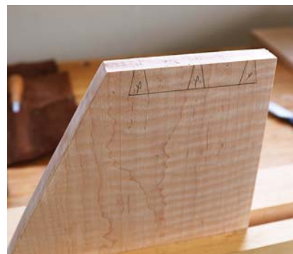
Tail board. On this build, the side pieces get the tails, with a half-tail on either end so as not to ruin the curve on the front, and to match it at the back.
