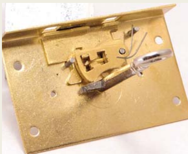
Ready to engage. With the main lever set under the openings in the selvage, the key is positioned to unlock or open the lock.
