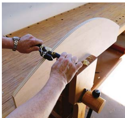
Shaving fair. A sharp spokeshave (followed by sandpaper as needed) made quick work of fairing the pattern's curve.
