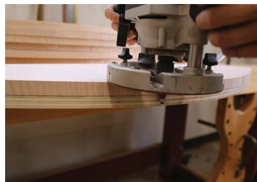
Rout to shape. Move at a steady pace as you guide the router around the pattern, and be sure to keep the base plate firmly on the workpiece.
