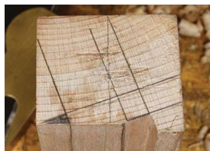
Double-check. There should be a gentle arris between the bevel face and the tongue face. Pencil the line to verify that it's straight and parallel along the length of the sole.
