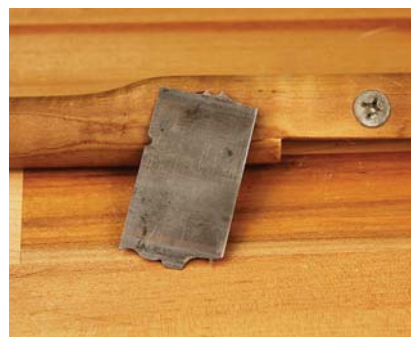
Scraper shapes. The most common moulding created with a bearer is a bead, but other profiles can easily be created as well.
