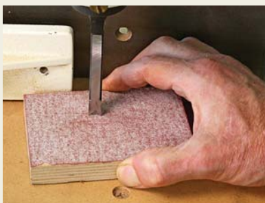
Only if you have to. If one of the points is damaged, you can grind the others down to match. If they are of equal length, skip ahead to the next step.
