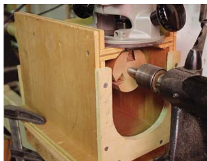
Dovetail jig. When attaching legs to turned columns, this jig proves invaluable.
