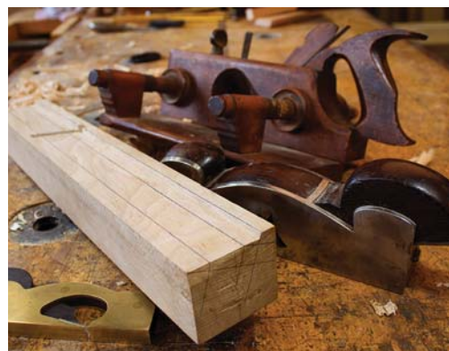
First profile cut. Use a wide moving fillister plane, shoulder plane or a rabbet plane to cut the square rabbet to the scribe lines on the heel, toe and right cheek.
