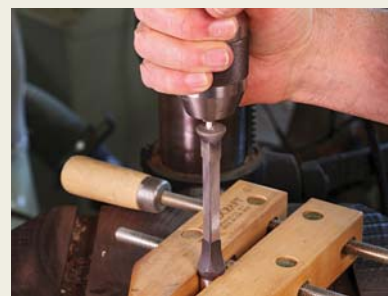
Alignment only. The sharpening cone can be placed in the drill press to keep it in line with the chisel. A few twists by hand are all it takes to hone the inner surfaces.
