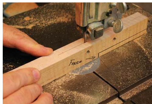
Cut the bearer. Saw a kerf through the end of the bearer that will hold the cutter. Make sure it passes both bolt holes to ensure adequate clamping pressure.
