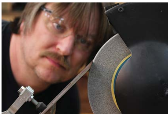
Setting the angle. When setting up to grind an iron, sight in from the side to keep the grinding centered on the existing bevel of the blade.
