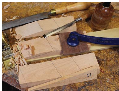
Wedge beginnings. Affix the wedge stock at the bench on top of a waste piece, then chop and pare the taper to your layout lines.
