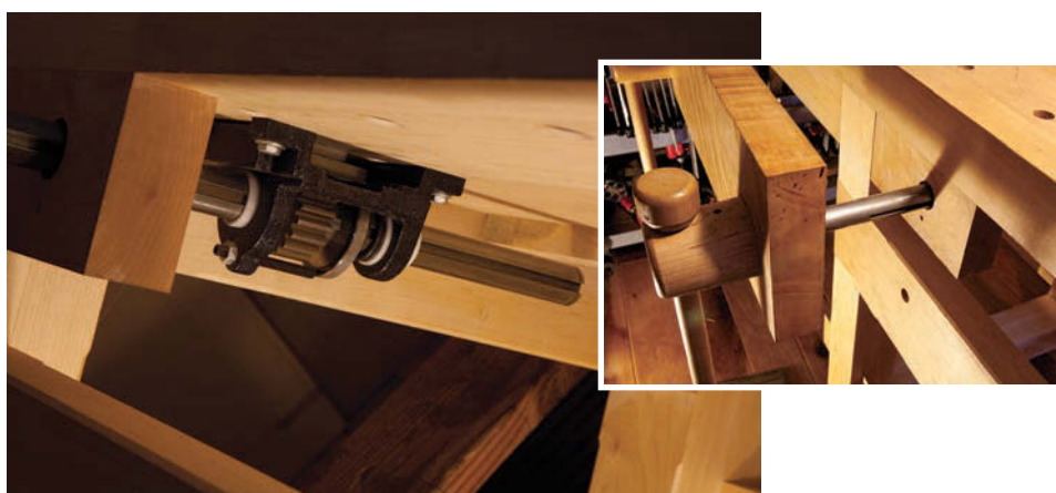
Hovarter Single Handle Face Vise. This Hovarter twin-screw opens and closes with a push or a pull. And it locks by twisting the handle clockwise a bit. It's a remarkable piece of engineering.
