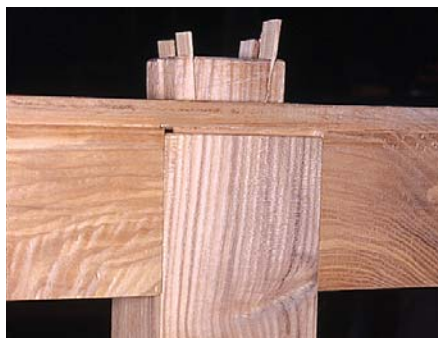
No turning back. This completed leg-to-beam joint is not going to work loose under stress. Once the wedges are glued in place and the extra tenon length is trimmed, the joint is pleasing to the eye and strong.
