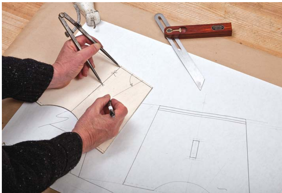
Divide and conquer. I often create a thin plywood template to represent components with angles and/or curves. The end boards of this step stool have both. To avoid the tedious and error-prone measuring process, I transfer all the dimensions from the drawing to the template using a pair of dividers.
