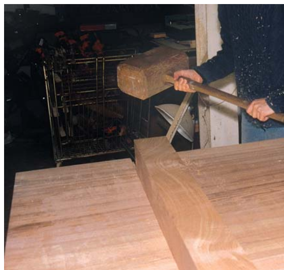
Aye, aye, commander. Dry-fitting a sliding dovetail into the table's tapered pin groove takes a big hammer – and a steady eye as you swing.
