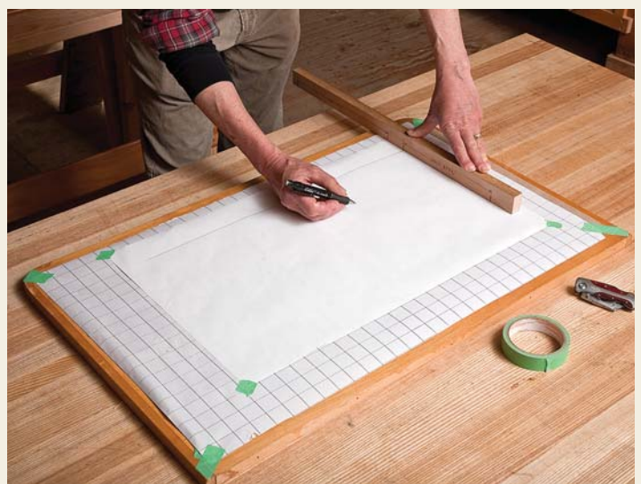
Simple needs. My drawing system is simple: a sheet of vellum spread over graph paper marked with 1" squares. By following the underlying crosshatch of lines I can easily create straight lines and right angles. Note that I'm using a tick stick to transfer the "hand-span" dimension to the drawing.
