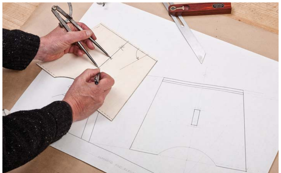
... then move the divider to the centerline drawn on the template.
