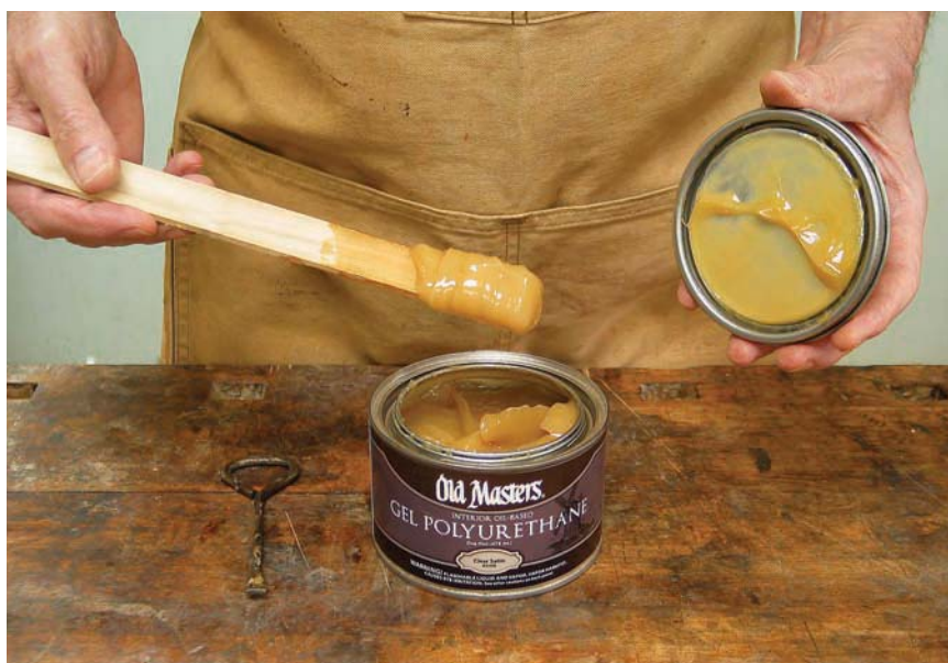
Thickness. Gel varnish is thick in the can, but it spreads easily because of its thixotropic quality.
