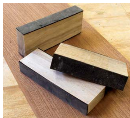
Careful clamping. Rubber-padded cauls are used to prevent clamp marks on routed edges.
