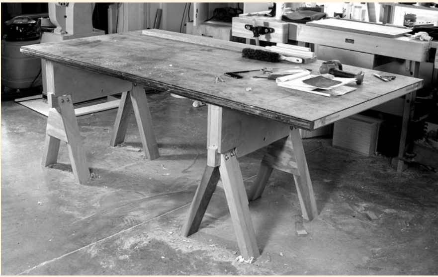
This rig serves as the assembly bench in the Popular Woodworking shop, but if you put a vise on it somewhere, it probably could serve as a workbench in a production shop. It is simple and allows great flexibility for clamping. But some basic operations with this setup would be tricky.
