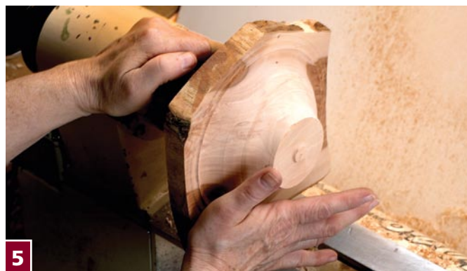
You should check occasionally to be sure the workpiece hasn't loosened on the mount. Screws can pull loose if they are in a softer spot in the wood. Stop the lathe, touch both the faceplate and the workpiece with a finger of your left hand, and give the piece a sharp tap with the heel of your right hand. If the piece has loosened, you will be able to feel it with your left hand.
