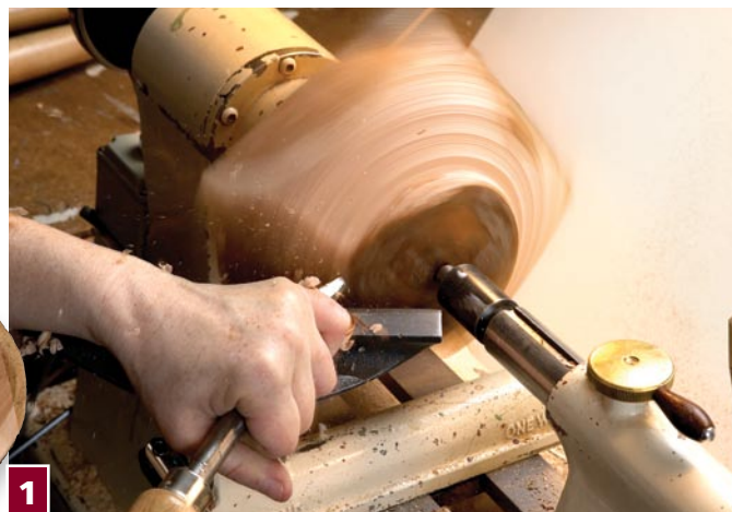
The workpiece is mounted with a faceplate screwed to what will be the top of the bowl. Use the tailstock for extra support while roughing out; a piece like this may be quite out of balance throughout the turning. With a side-grind bowl gouge, turn from the bottom toward the rim with the flute (groove) pointing in the direction you are turning, and cut with the edge just to the left of the center of the tool (the lowest part of the edge).
