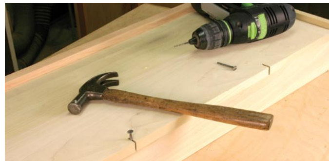
Two slots cut in the drawer bottom just to the inside of the drawer back is where the nails are set to hold the solid drawer bottom. The slots allow for seasonal adjustments.
