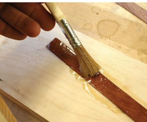
Hide glue is generously applied to the back of the edge veneer with a brush.
