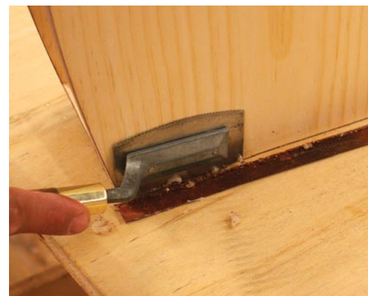
Let the glue cool and stiffen, then use a veneer saw to trim off the excess. You should leave 1/32" to 1/16" margin.
