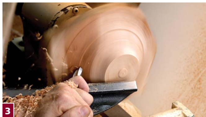
Continue shaping the outside of the bowl. Here you can see exactly how the gouge is cutting. Keep the bevel riding on the wood behind the cut. That's how you keep control of the tool and the cut.
