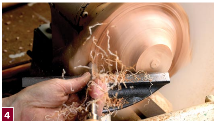
If the rim is turned downward, as mine is here, you will need to reverse the direction of the tool motion on that part. Push the tool into the cut, not toward the workpiece itself, and blend into cut you made from the side. (Also, see "A Familiar Tool" on page 93.)
