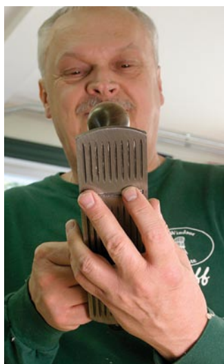
Use your fingertips to ensure the blade is centered in the mouth and projecting enough to make a cut. Test your setting on a scrap of wood.
