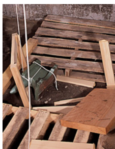
The cube made from biscuits after impact.
