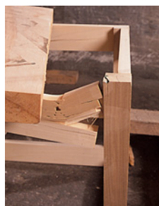
The mortise-and-tenon cube after the first hit.
