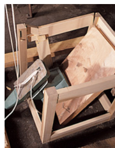
The mortise-and-tenon cube after the second hit.
