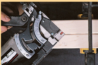
You can biscuit miters without using your fence by clamping the two joints together.
