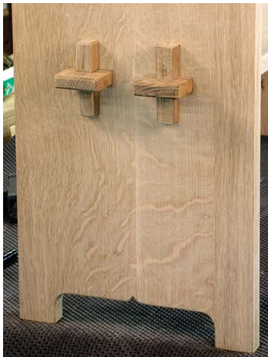
Hard & soft. Edges on the tenons and keys are beveled, but they fade away to leave clean lines at the joints.
