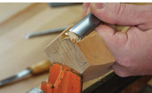
Middle toe. Invert the 20mm No. 5 gouge to shape the front toe.
