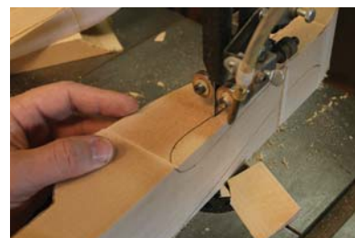
Cut the leg. Cut out the cabriole leg using the method you like (my “Cabriole Legs Simplified” DVD offers good instruction).
