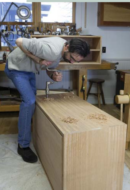
Holes & pegs. The 1½" holes were bored using a modern Forstner bit and a brace (yup, that works). Before inserting the dowels into each hole, the ends were chamfered a bit to make the units' docking procedure easier.
