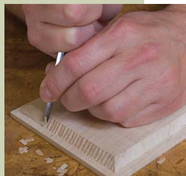
Smooth motion. Start at the field edge; take a light cut down the slope and ease up as you reach the bottom.
