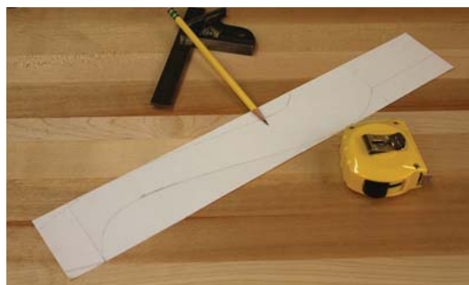
Draw the pattern. The cabriole-leg pattern doesn't vary much from a pad-foot pattern.
