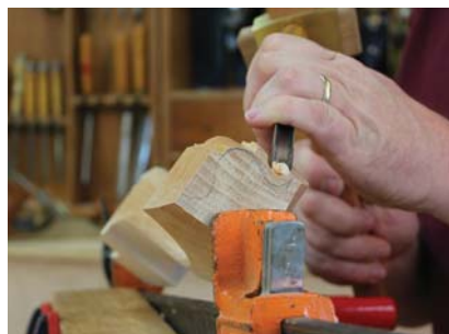
Toe jam removal. Use your 12mm No. 9 gouge to remove the bulk of the waste between the toes.
