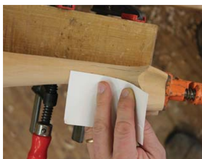
Upper marks. Using poster board as afflexible straightedge, mark the upper portions of the center toe.
