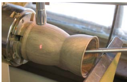
Hollow the inside. A laser (note the red spot on the side) tracks the location of the tool deep inside the box and makes it simple to hollow.
