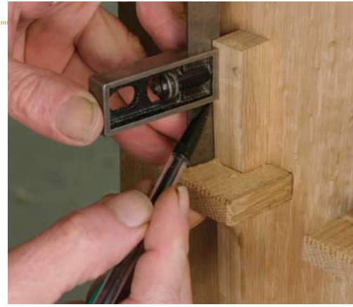
Fit first. Leave the wedges long until they fit nicely in the mortises, then mark and cut them to length.
