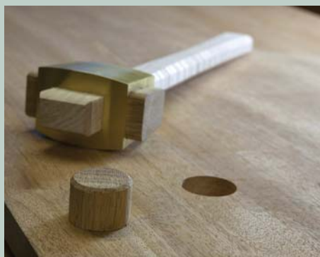
Holes & pegs. The 1½" holes were bored using a modern Forstner bit and a brace (yup, that works). Before inserting the dowels into each hole, the ends were chamfered a bit to make the units' docking procedure easier.
