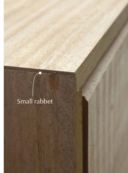
Full blinds. Here are the dovetails for the secretary's top. Note the small rabbit at the end. When the joint is assembled the rabbit is the only part of the joint that shows.
