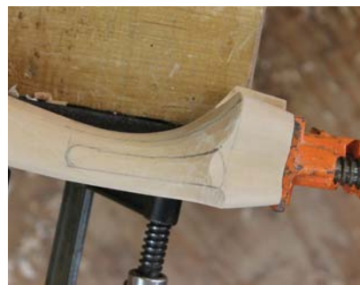
Cove. Mark out the cove for the webbing between the toes.
