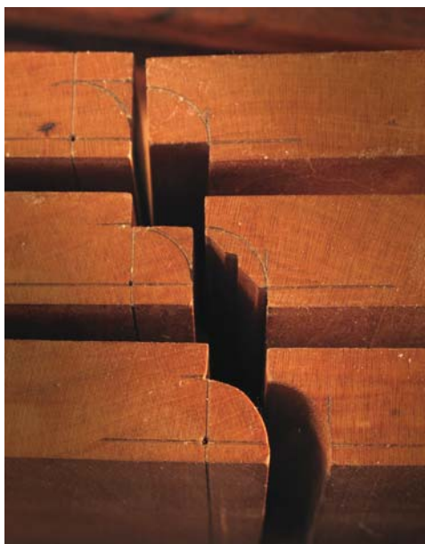
Work down with hollow & round. Use a rabbet plane to establish the fillet and land. Then finish shaping the joint using hollows and rounds.
