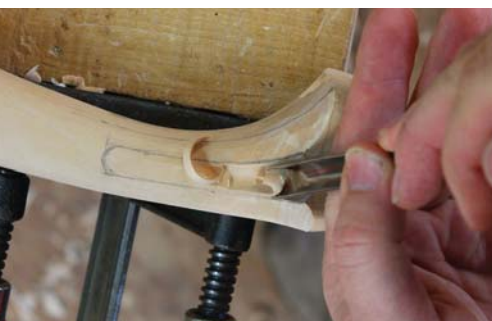
Carve. Using a 12mm No. 9 gouge, carve to the lines.
