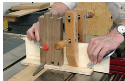
Careful aim. The blade cuts a slot in the bottom of the fixture; use that to line up the cuts before clamping the parts.
