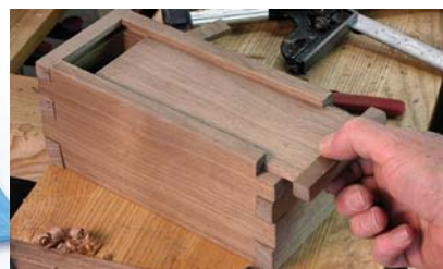
Visual aid. The line of the joint helps to reduce the visibility of the junction of the top and bottom.
