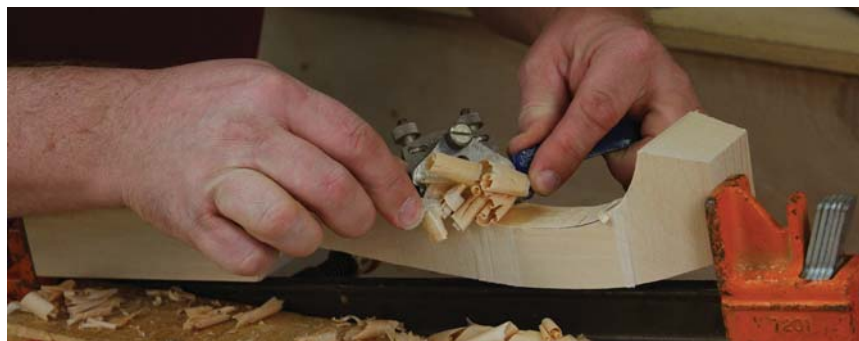
Refine the shape. Smooth, shape up and refine the curves on the leg using a spokeshave.
