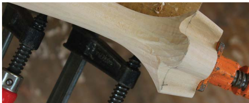
Foot one. The simple trifold foot – the basis for variations two and three – is now ready for sanding.
