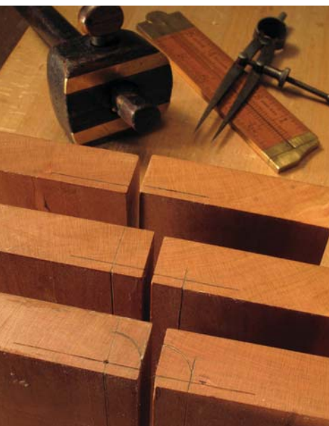
Mark out for hollows & rounds. Scribe layout lines on the ends and faces of the stock to guide the planes
