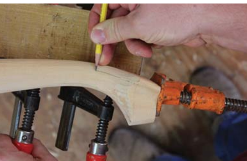
Finger guide. Use your finger to extend the toe line up through the ankle of the leg.
