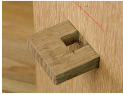
Just behind. The square end of the mortise lies behind the face of the side to allow the wedge to seat tightly.
