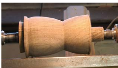
Turn the outside. The first step is turning the outside shape with the blank mounted between a spur center and a live center in the tailstock.
