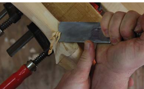
Height. After marking off the height of the foot at about 1\frac{1}{8} ", use a bench chisel to bring the foot to final height.
