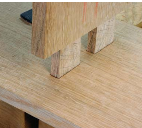
Ease in. Bevel both the ends of the tenons and the edges of the mortises for fitting.
