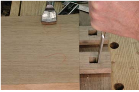
Angle by eye. Use a chisel to taper the end of the mortise for the wedge.
