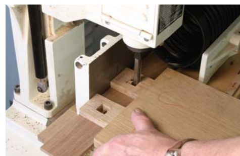
Back it up. A thin piece of scrap under the tenon provides support when making the second mortise.
