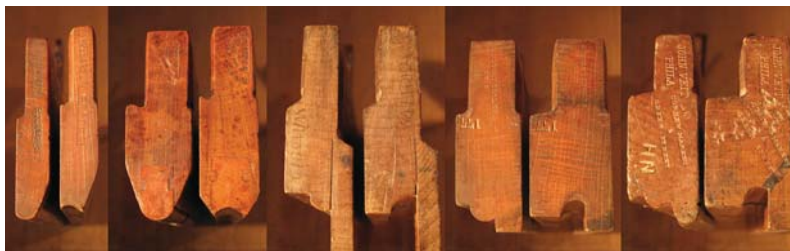
Take your pick. Rule joints can be cut using either a set of hollows and rounds, like the set at left, or with a matched set of table joint planes, like the four other sets shown.
