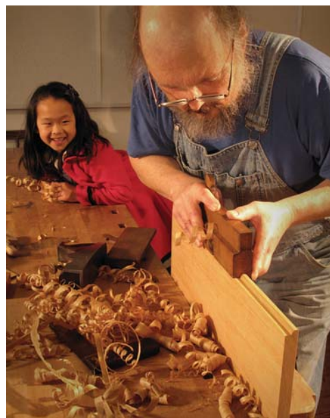
Or use dedicated planes. Matched sets of table joint planes cut perfectly matched profiles – simply work to a scribed line.
