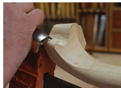
Curve. Round over the hard edges of the outside toes.
