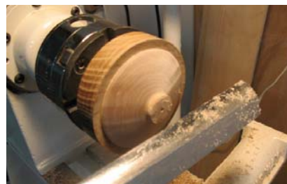
All jammed up. Once the lid’s inside is done, the lid is mounted in a jam chuck to turn the outside.
