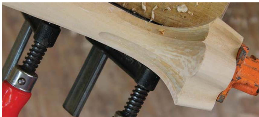
Foot two. The webbed trifid foot variation is now ready for sanding.
