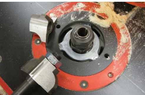
Router better rule joints. For period-looking machined rule joints, choose a set of bits that cuts a rule joint with a \frac{3}{8} " radius.
