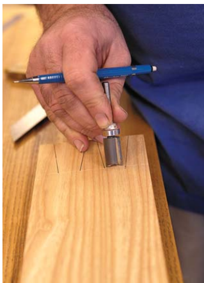
Leave a space. Size your tails so the base is wider than the router bit's diameter.
