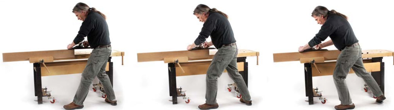
Freedom to control. When the arms and hands don't do the heavy work, those muscles are available to control the position and pressure of the tool.
