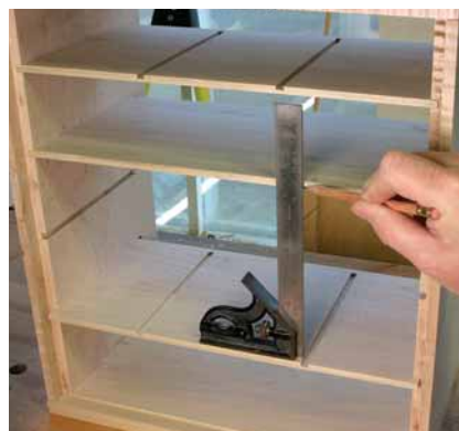
Accuracy is a must. Keeping dividers square to the shelf is best done using a combination square. Align the square's base to pinpoint the opposite dado.
