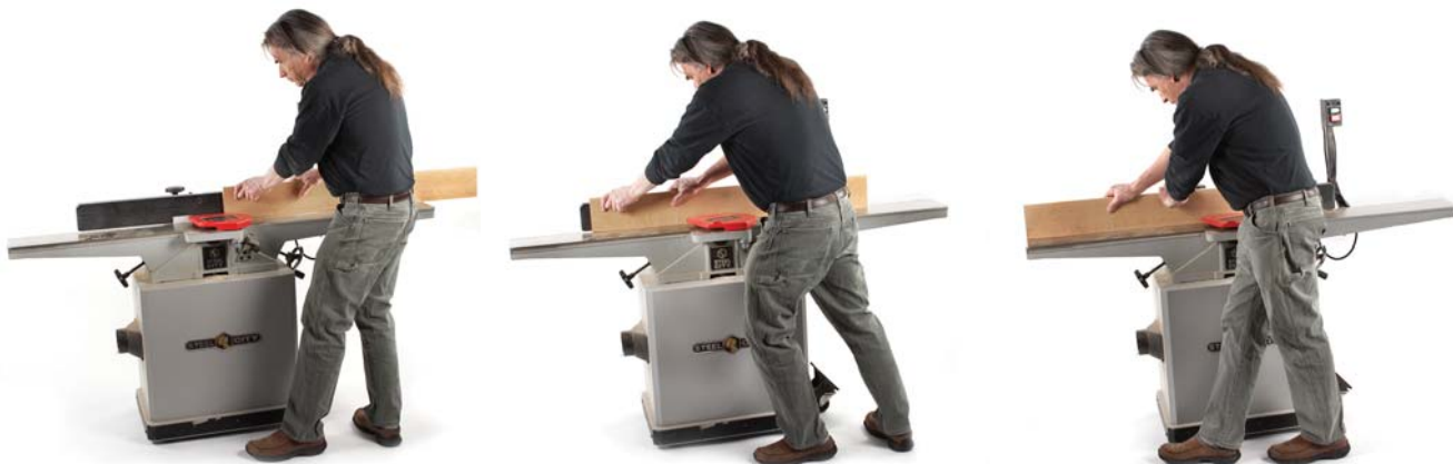
Power tools, too. Shifting weight to provide motion provides consistent control at the jointer, as the feet take a step and walk through milling an edge.
