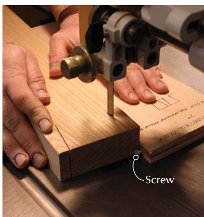
Mirror image. Flipping the board cuts the opposite tail perfectly without measuring.
