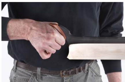
Get the point. Extending the index finger makes aiming and controlling easier. It also changes the angle of the wrist to make movement effortless.
