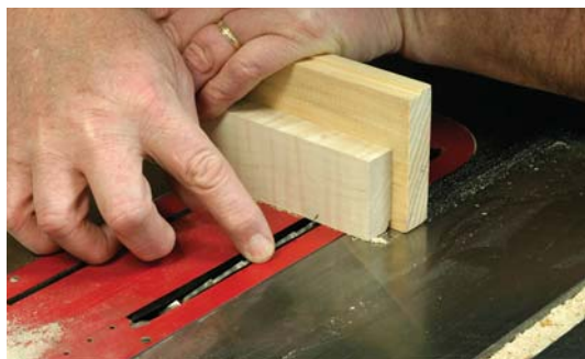
On the right side. Cuts to define the mitered sticking should be on the waste side of your line, or in the stile area. Make sure to use the correct blade tooth when setting the cut.
