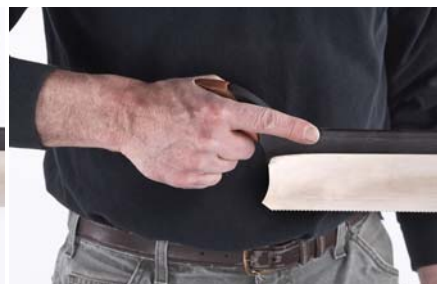
Get the point. Extending the index finger makes aiming and controlling easier. It also changes the angle of the wrist to make movement effortless.
