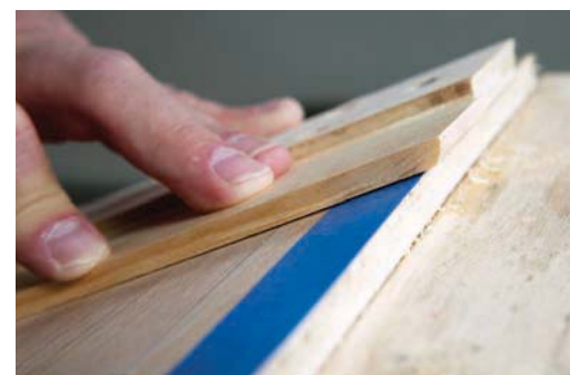
Tape trick. You can increase your board's precision by using a strip of painter's tape to lift (as shown) or lower the angle.
