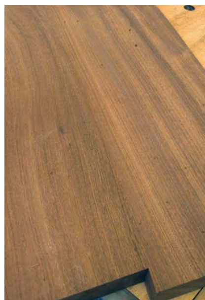
Where's the joint? Two routed edges, joined together, produce a tight, clean and nearly invisible seam.
