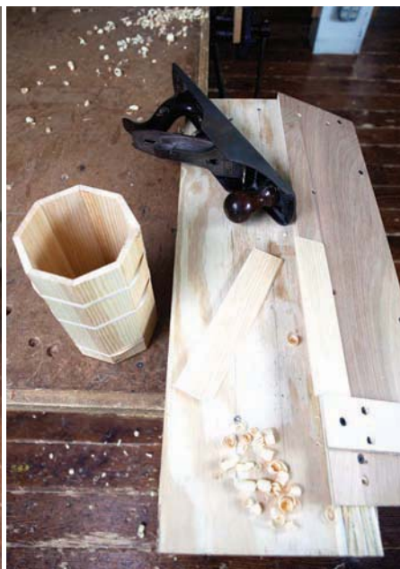
Donkey's ear. A 45° donkey's ear is used to trim standing miters and edges. For coopered work, make a board at another angle. The one on the right is 22½° and makes an octagonal form.
