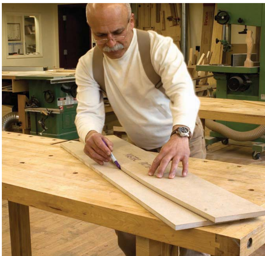
Pattern repeat. After fine-tuning the master pattern outline, transfer it onto a wide piece of 1/2" MDF.
