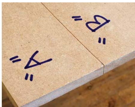
Pattern repeat. After fine-tuning the master pattern outline, transfer it onto a wide piece of 1/2" MDF.
