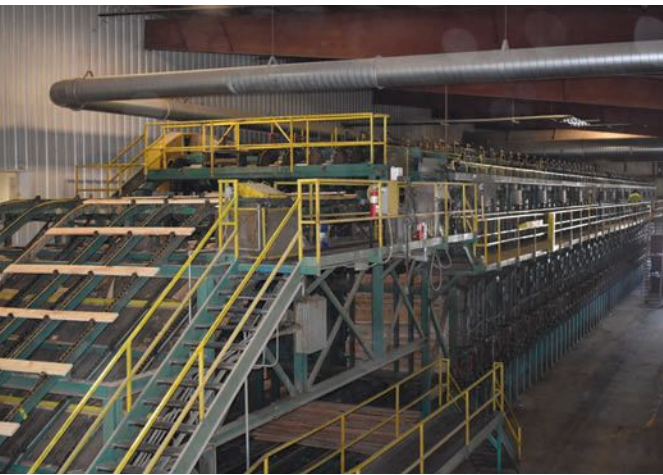
Granite Valley Forest Products has a 60-bay bin sorter, allowing for custom sorts based on length, width and color.
