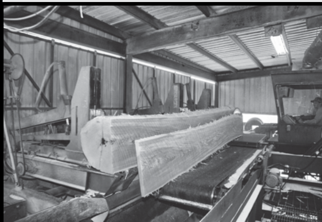
This is an inside view of one of Kepley-Frank's sawmills cutting a large log. The firm cuts lumber in 4/4 through 8/4 thicknesses.
