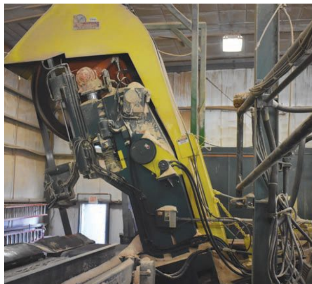
Granite Valley's AAA Hardwood facility operates a 6-foot McDonough headsaw with a 17-degree slant.
