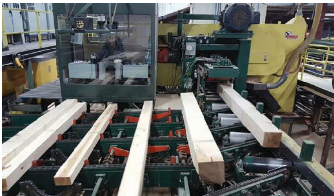
Wheeland Lumber Co. Inc. in Liberty, PA, runs this automatic feeding MAXX Infeed on a McDonough horizontal resaw system.
