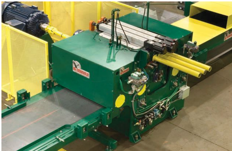
This is an overview of McDonough's linear edger in their equipment manufacturing facility.
