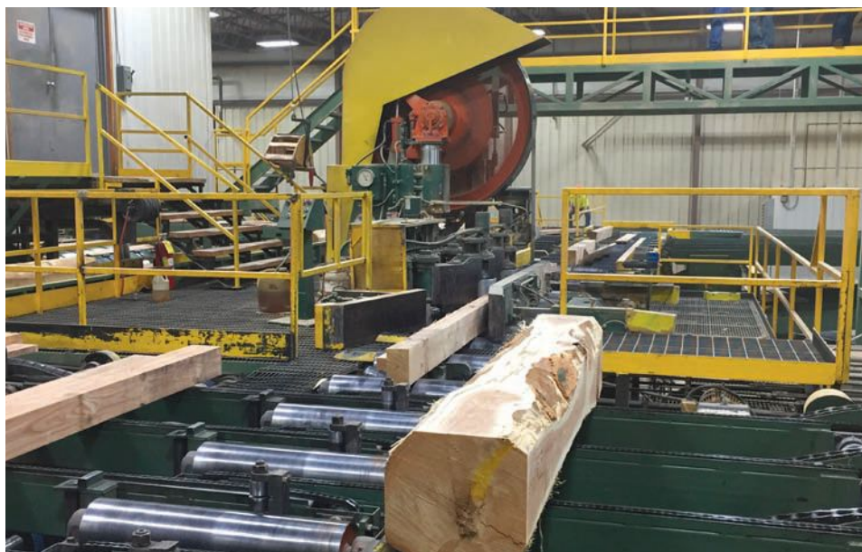
Quality Hardwoods in Sunfield, MI, installed this 6-foot McDonough linebar resaw for sawing Hardwood cants.
