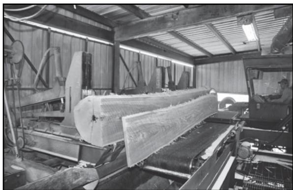
This is an inside view of one of Kepley-Frank's sawmills cutting a large log. The firm cuts lumber in 4/4 through 8/4 thicknesses.
