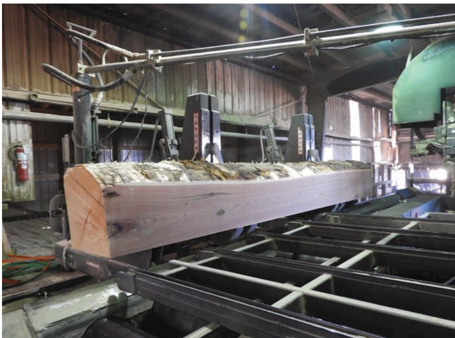
This view inside the company's mill facility shows G.F. Hardwoods' Letson & Burpee high-strain saw in action.
