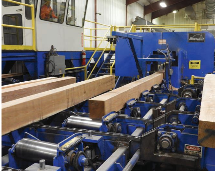
Cants continue through the process being cut by a Brewco resaw at the Tamworth facility.
