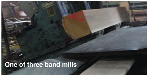
Cants being sawn into lumber at the resaw
