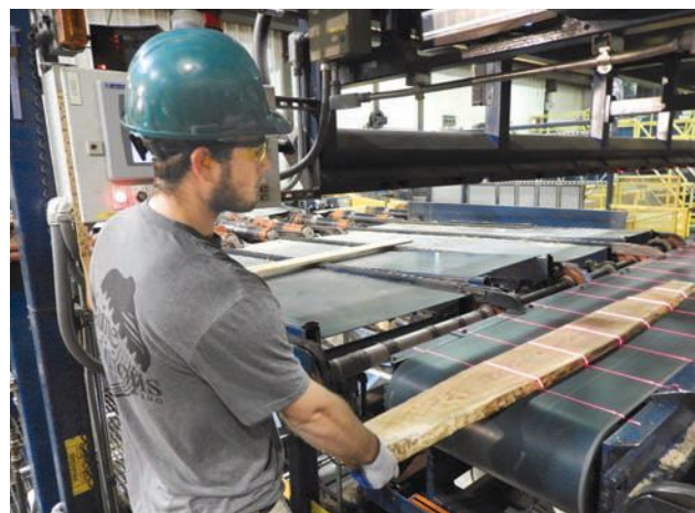
A Kennebec worker puts a board through scanning prior to it entering the 3D edger with wiggle box technology.
