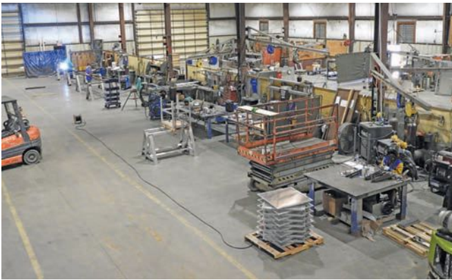
SII's spacious welding shop is where fabrication of dry kilns is accomplished.
