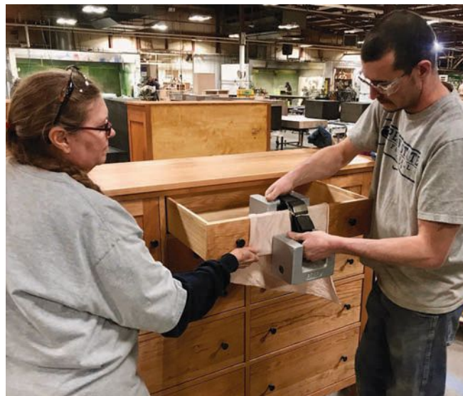
Stability testing is conducted to qualify specific Gat Creek designs as Product Stability Verified.
