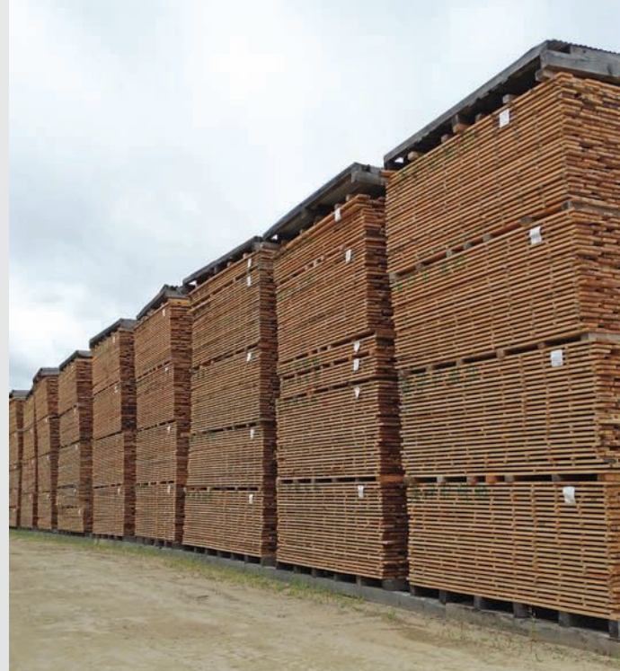
Abenaki Timber provides quality air drying with pile tops.
