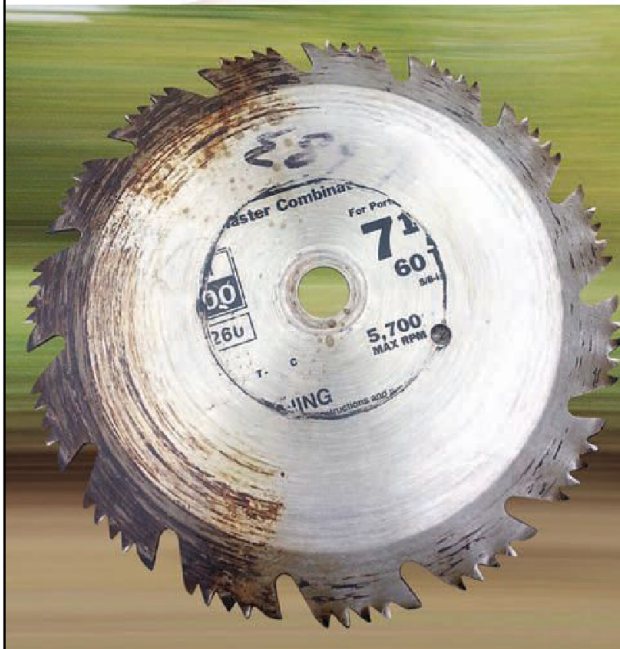
Right side of blade cleaned with Lubie FC930.
