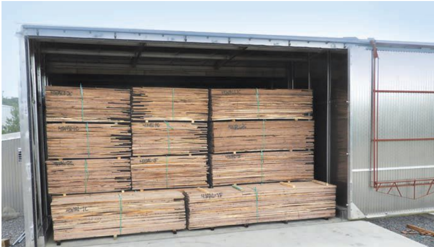
A new 55,000 board foot capacity Walnut steamer was manufactured and installed recently by A.W. Stiles Contractors Inc.
