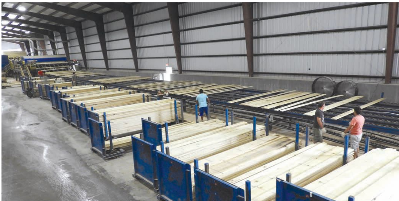
Cardin Forest Products added a new 47,000-square-foot facility to accommodate its state-of-the-art dry line, which is a material handling system by Froedge Machine & Supply Co. Inc.
