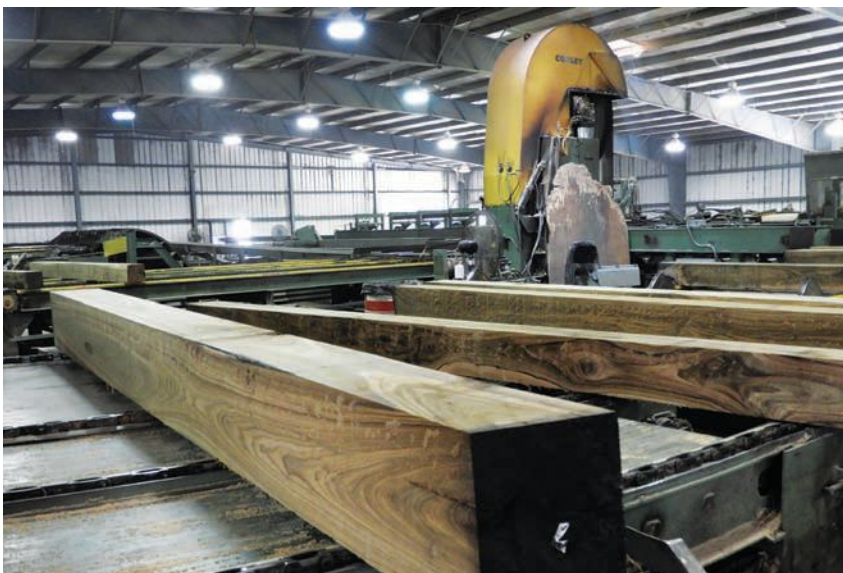
Walnut cants are being further processed into grade lumber by the 7-foot vertical band resaw.
