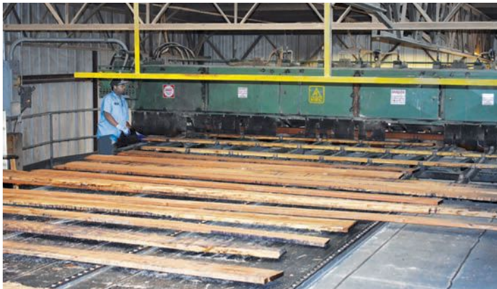
The company has an HMC multi-drop saw trimmer, which lumber passes through before getting graded and dipped.
