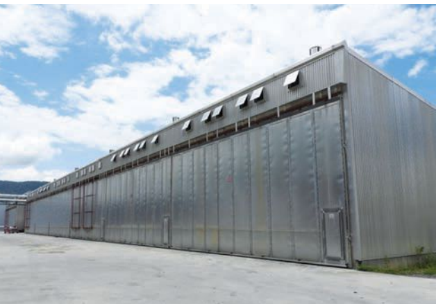
The company has nine dry kilns manufactured by SII Dry Kilns, with the ninth added earlier this year, giving Cardin Forest Products a total drying capacity of 900,000 board feet per charge.
