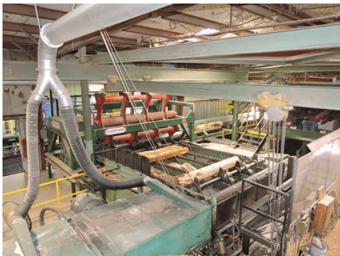
Pictured are logs at AJD being processed through a Cleereman Industries' Rotary Log Kicker.
