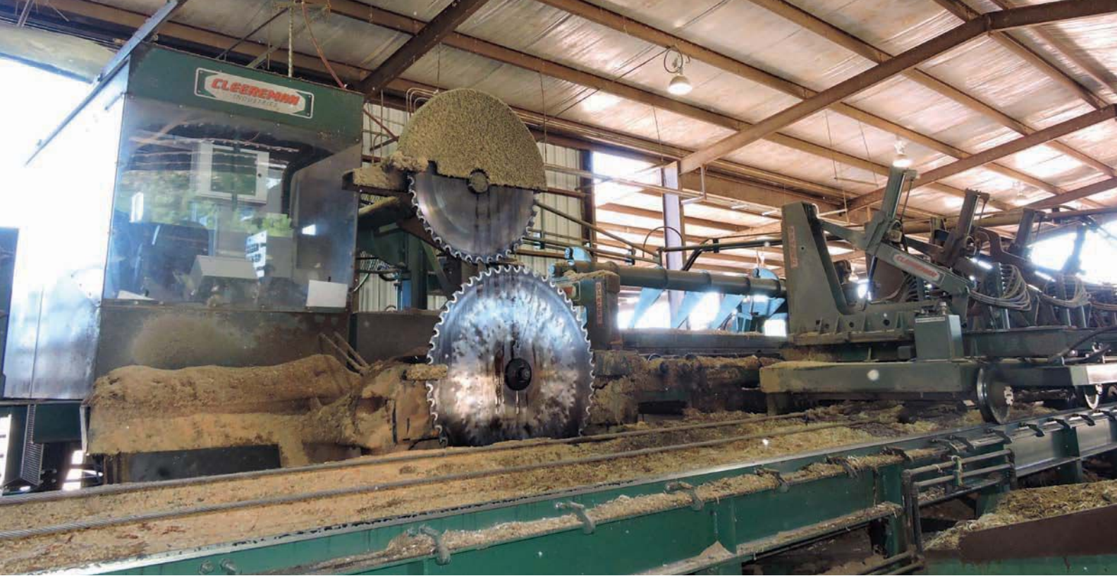
At Netterville, the new primary breakdown headrig by Cleereman Industries is pictured.
