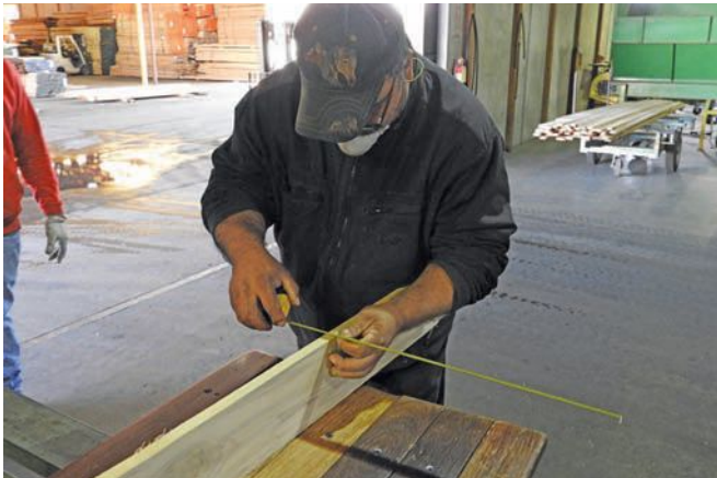
Accuracy and precision are most important at Sweeney Hardwoods. After setting up the planer, thickness is double checked before continuing with the order.
