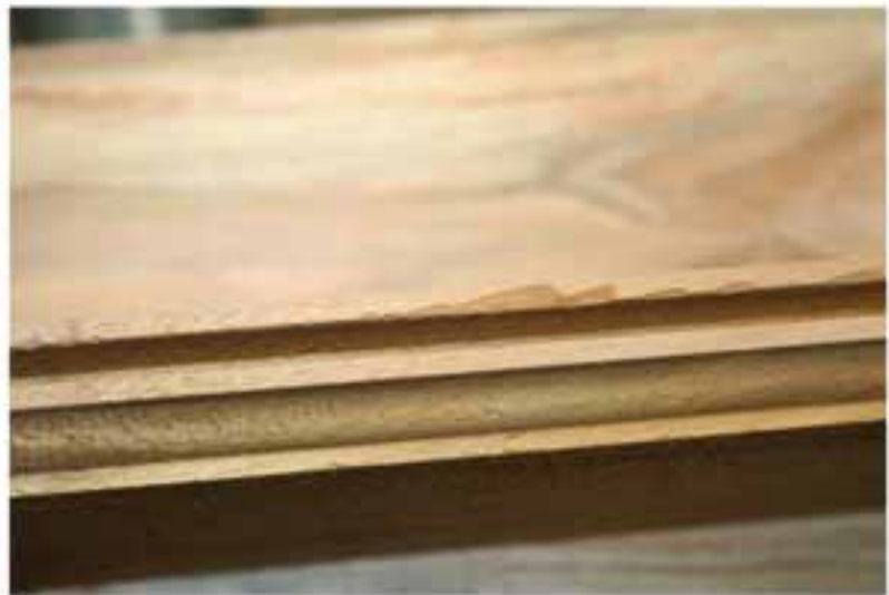
Chipping Defect produced [Pic 2]
