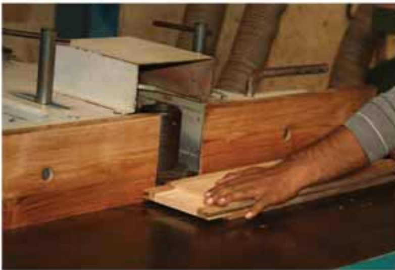
Defective operation [Pic 1]
