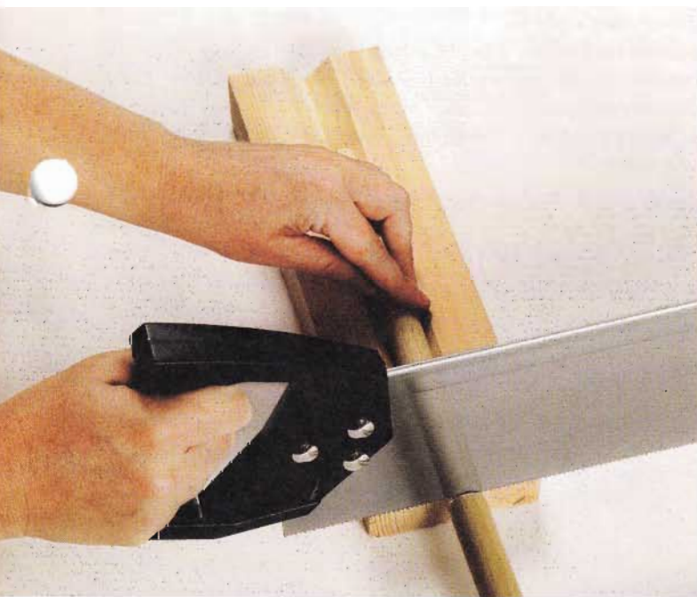
A V-block jig keeps round pieces from rotating during cutting.
