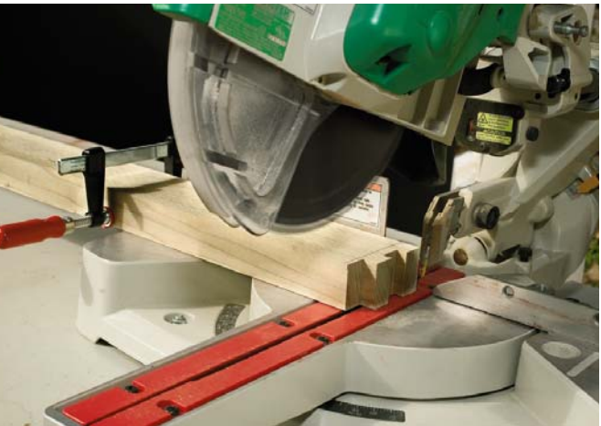
Gang cutting produces multiple identical workpieces.
