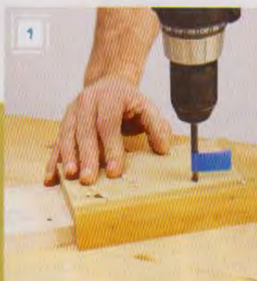
Use a piece of painter's tape as a flag to indicate the proper drilling depth when you drill the holes with the pin-hole jig.
