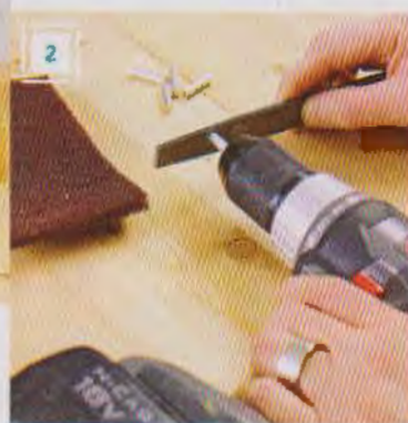
Chuck \frac{3}{8} " of each pin in a drill. With the drill flat on your bench for stability, spin the pin against a file. Buff the pin with an abrasive pad.
