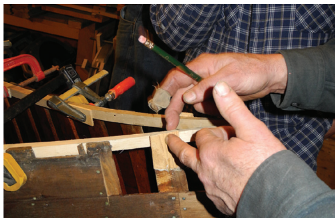
Bringing old wood and new wood together at the gunwale
