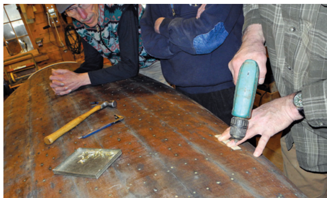
Fitting and installing patch
