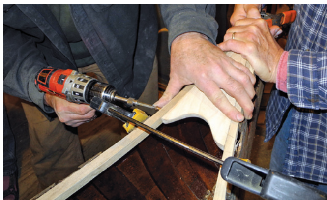
Installing the new "deck", also known as the "breast hook"
