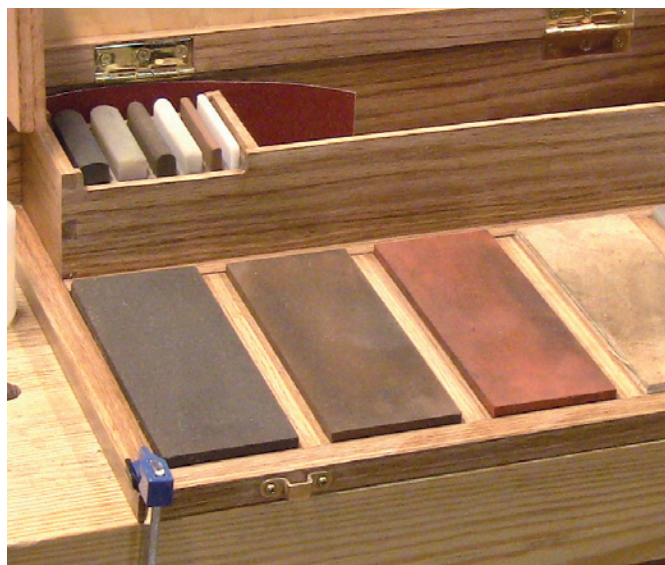
Portable sharpening station with oilstones and leather strop. This makes sharpening much more convenient.
