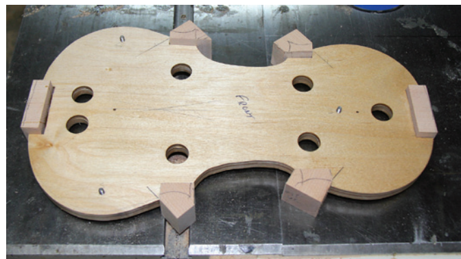
Corner blocks glued to form
