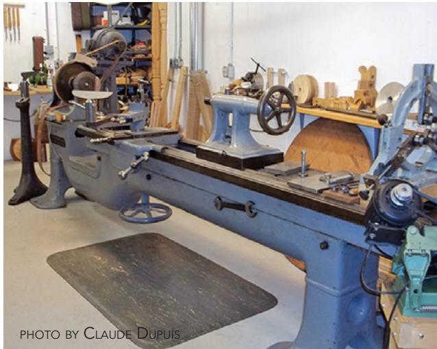
1900 Putnam extension-bed patternmaker's lathe (wood lathe), 50" swing inboard thru the gap
