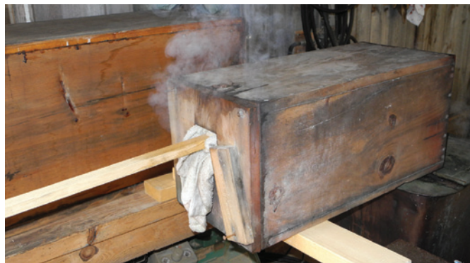
Steambox in operation. About 18 inches of a spruce inwale is being steamed so that it can take a sharp bent at one end
