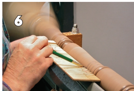
After reducing the diameter in the middle area, the marking jig is used for a second time (jokingly referred to as "making a remark").
