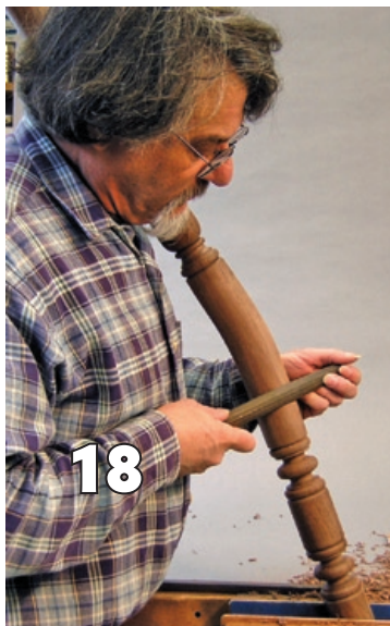
← A double-cut file further refines the surface.
