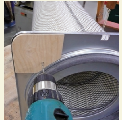
8—Fixture to drill 4 holes in the corners of the filter flange
