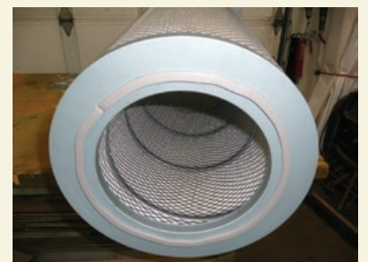
14—Closed cell foam between the two filters
