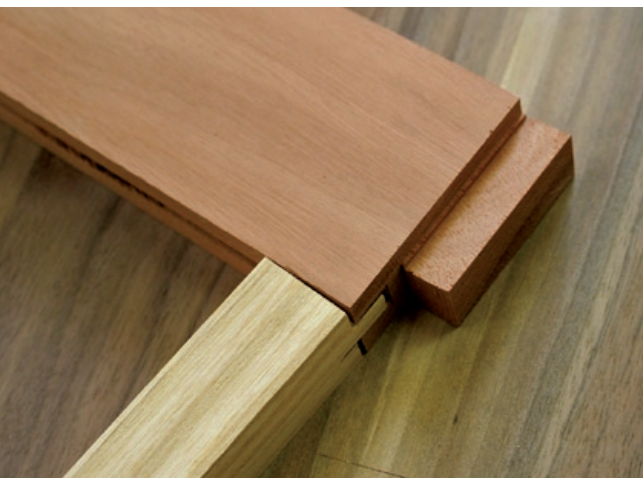
Dovetail divider with groove and mating runner
