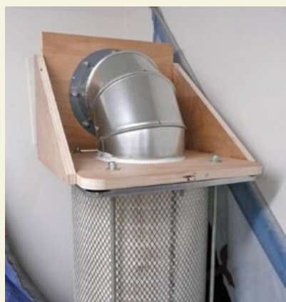
17—Upper half of filter assembly
