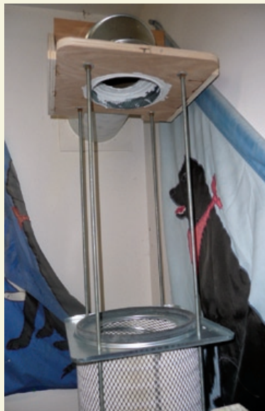
15—Assembly of filters to support bracket
