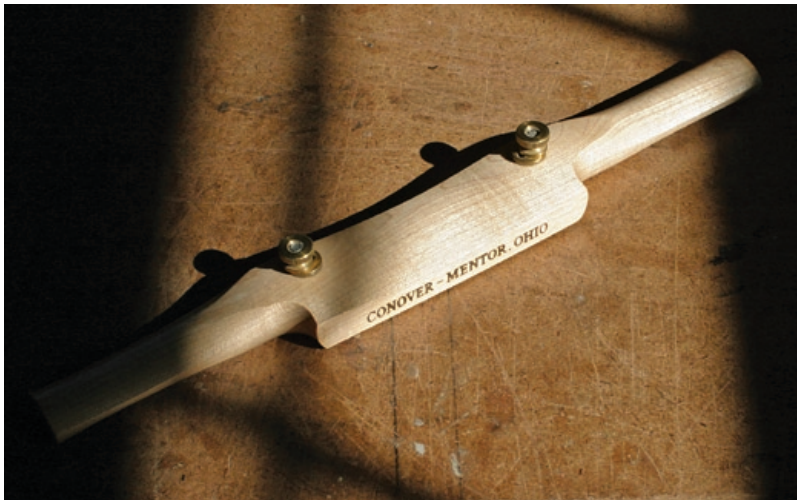
An example of Ernie Conover’s spoke shave with set screw adjustment and modified handle.
