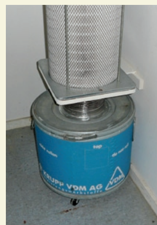
22—Dust barrel attached to the bottom of the filter assembly
