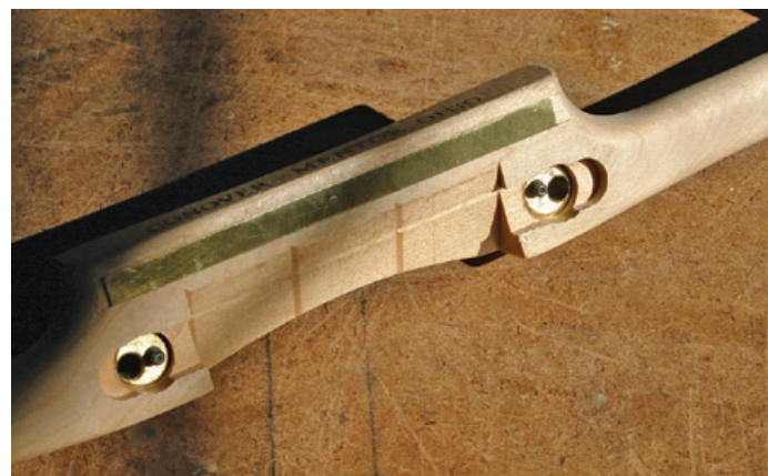
An example of Ernie Conover’s spoke shave with set screw adjustment and modified handle.
