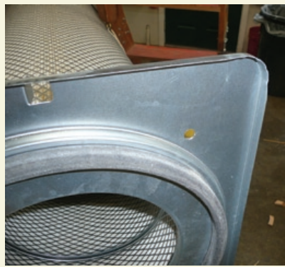
9—Step drill clearance for \frac{3}{8} " rod
