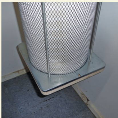
18—Lower half of filter assembly
