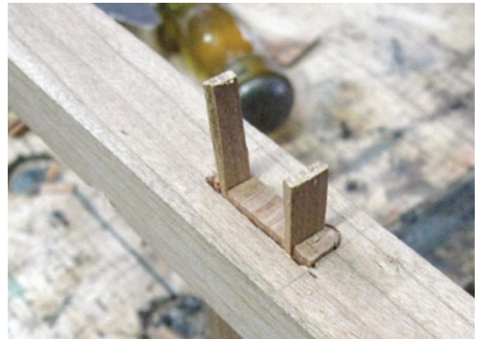
Wedges in place
