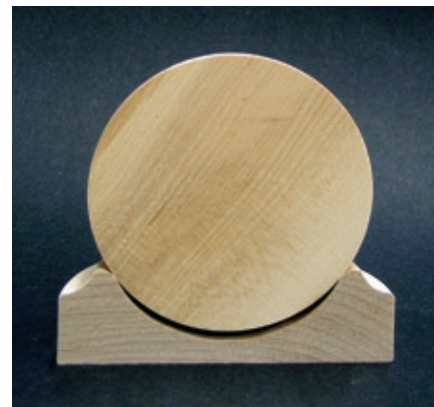
Cross section shows how the sphere seats in the cup chuck.
