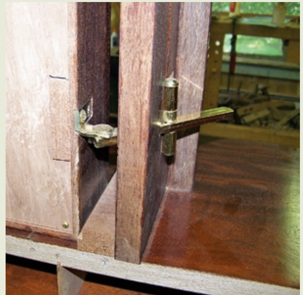
Temple hardware as connected to the inner painting mounting box.
