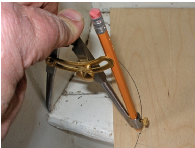
Photo #12 — Spiling Step #1
