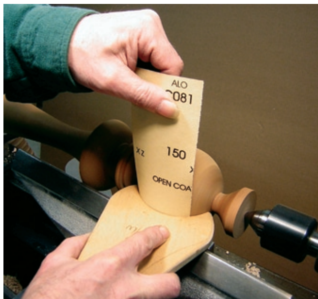
Lower the tool rest, and press the sandpaper against the ball with the template.
