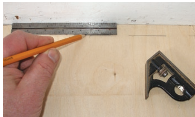
Photo #4 — Use of a straight edge
