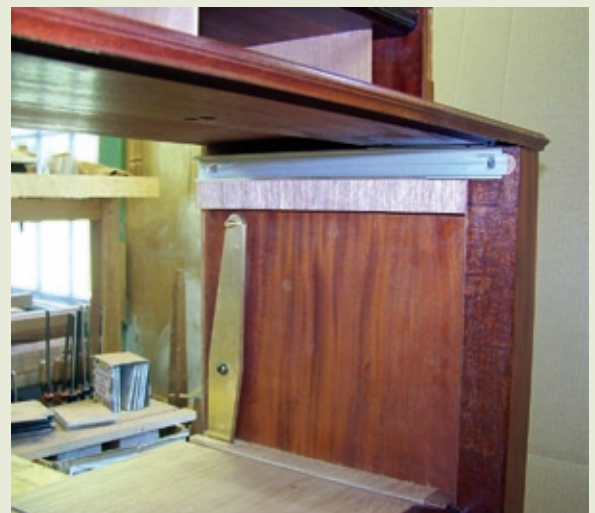
Showing lid/slide mechanism as located behind the front stile.
