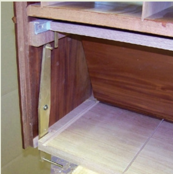
Lid/writing slide mechanism showing transfer of motion from lid at top to slide in lower case — it protrudes through the bottom of the upper case into the lower case.
