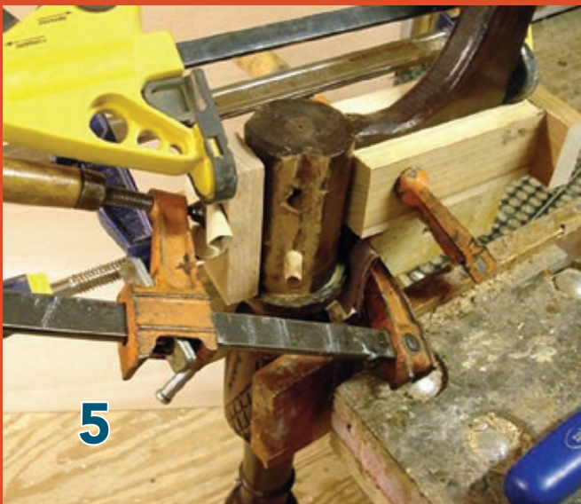
I glued and clamped each leg into alignment.
