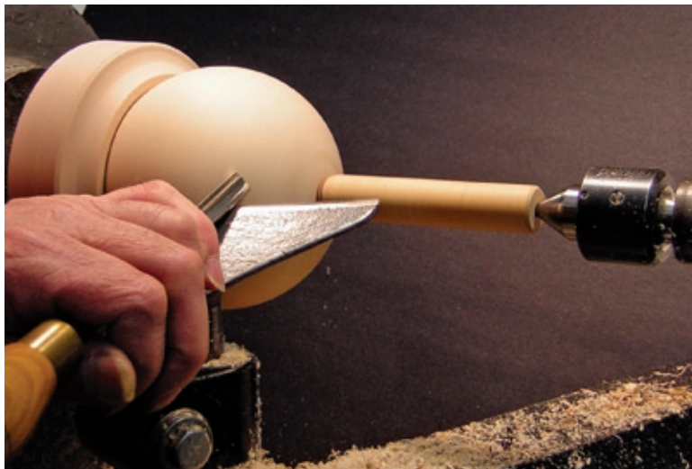
Final step in refining the sphere in a cup chuck.
