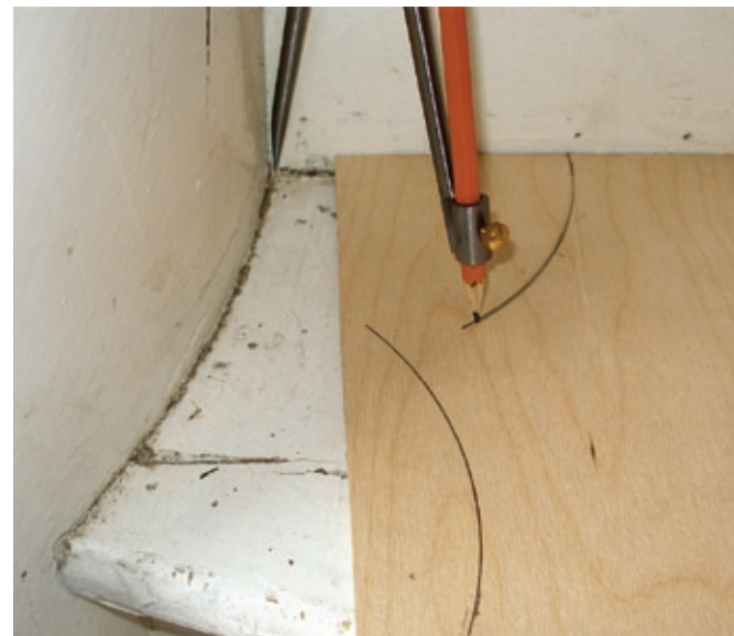
Photo #13 — Spiling Step #2
