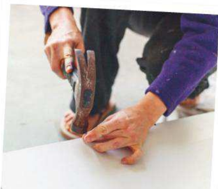
ABOVE MDF was attached to the sideboard to create a backing. BELOW Patched cut-outs were clamped while the adhesive dried.
