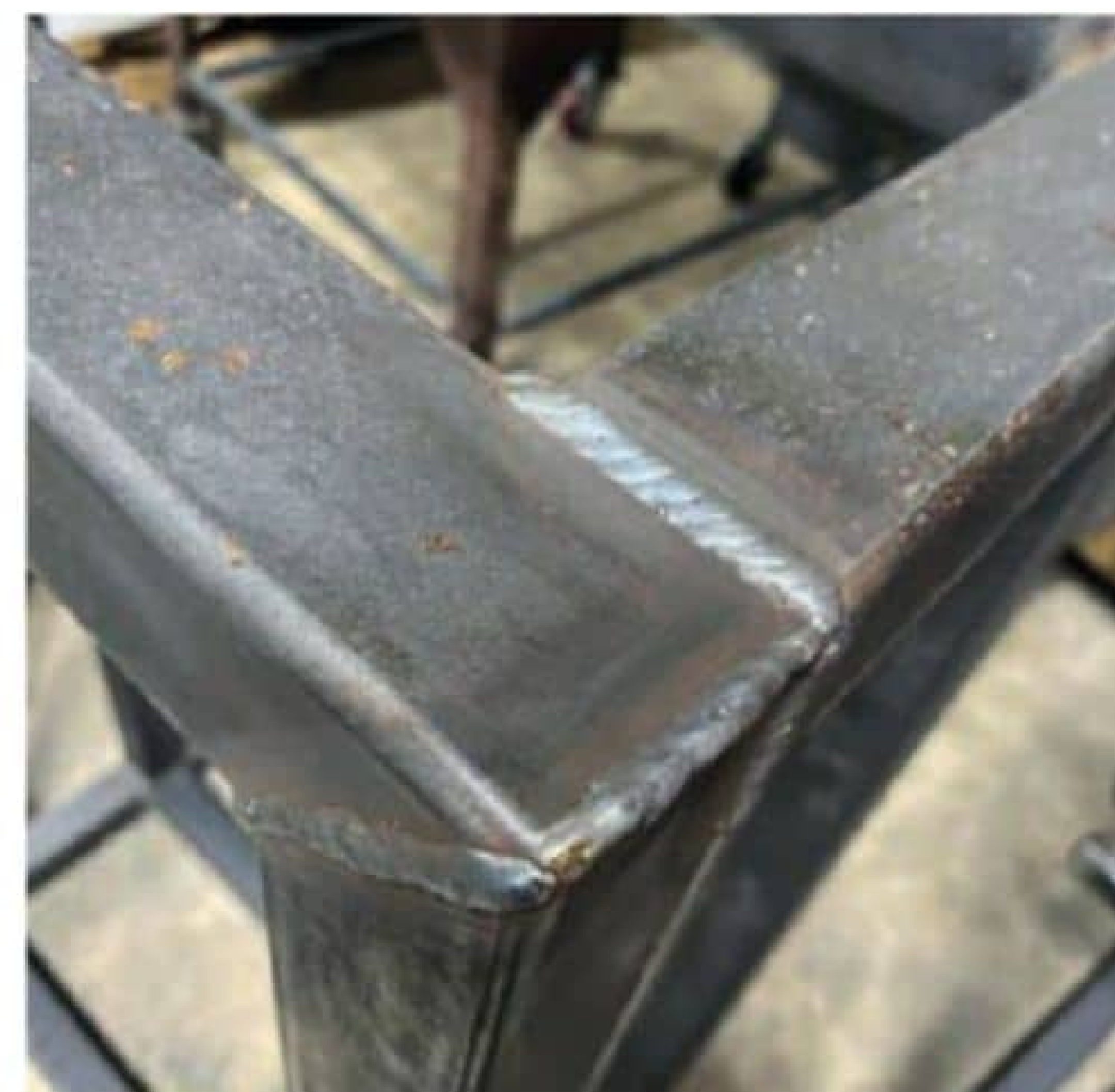
Carefully smooth down all welds
