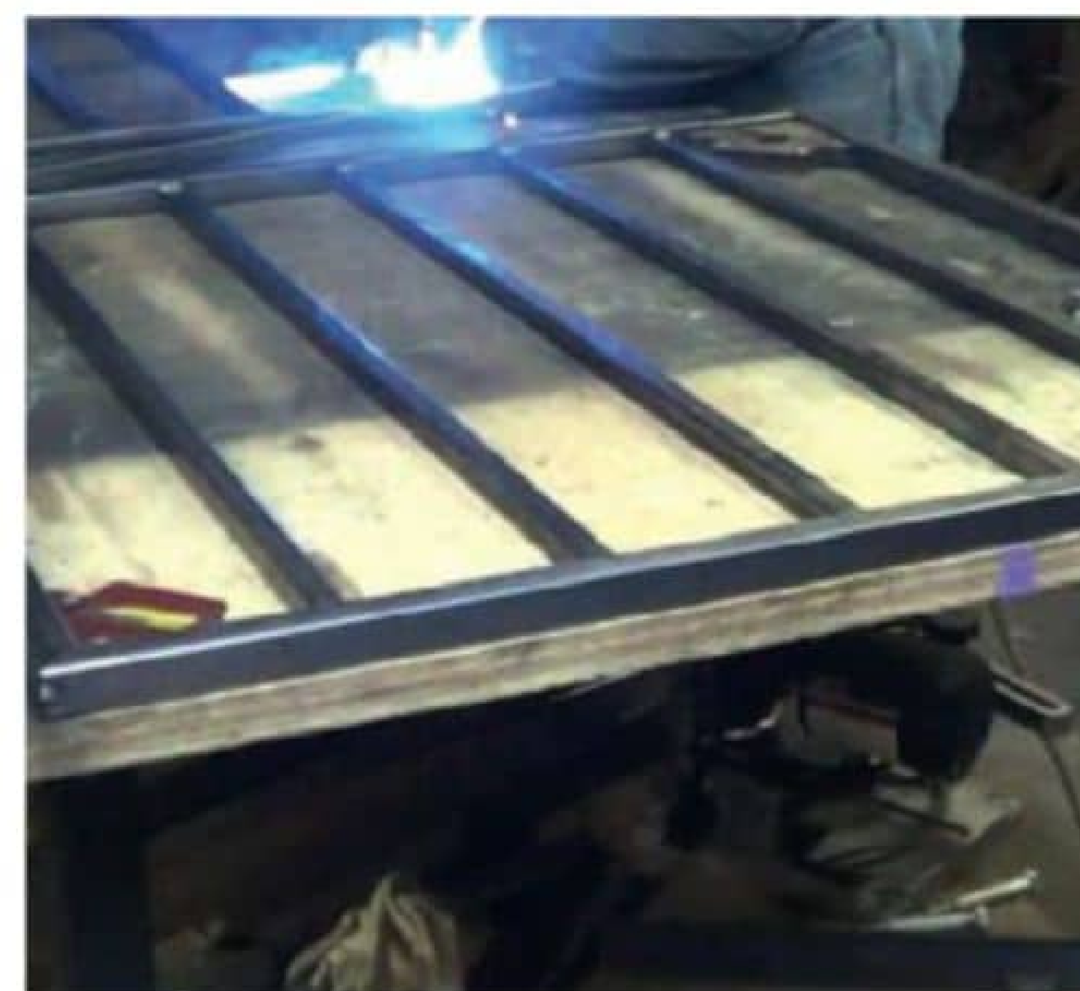
Space vertical bars 80 to 100mm apart
