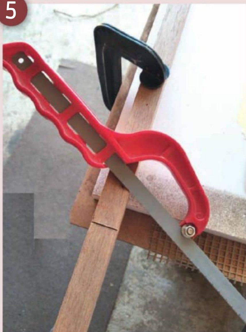
Cutting with the hacksaw
