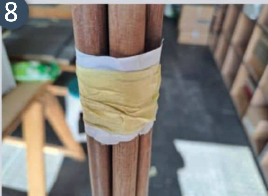
Masking tape not touching dowels
