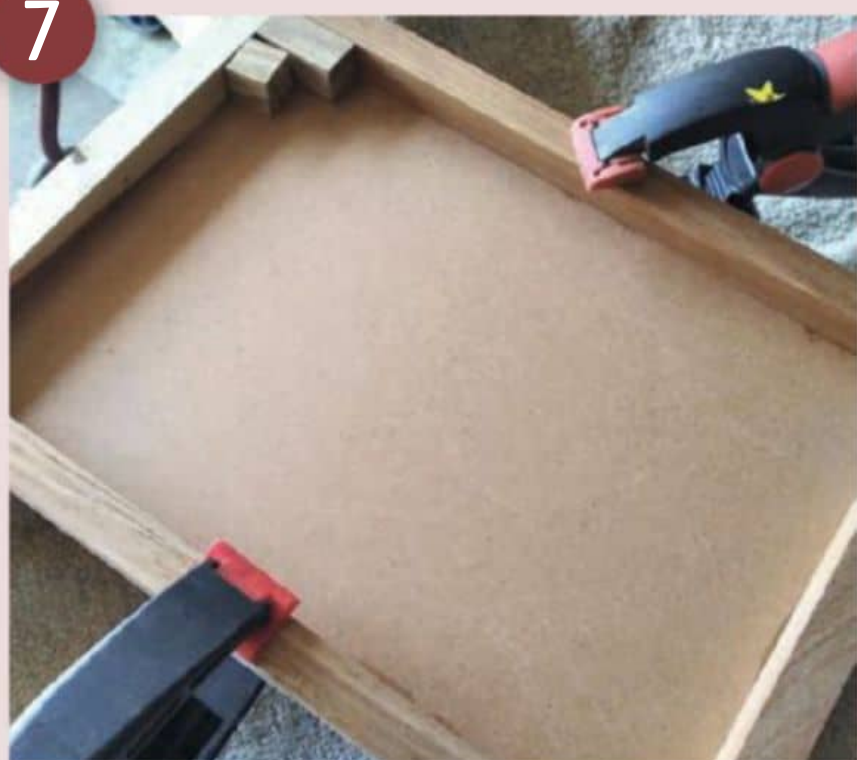
In this picture, I'm using the spring clamps to hold the frame in position
