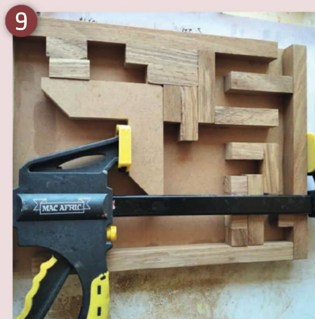
Aligning and clamping using a bar clamp
