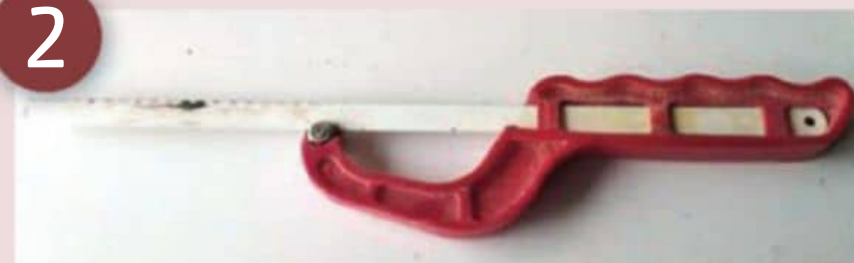
Hacksaw blade Holder with blade fitted teeth facing towards the handle
