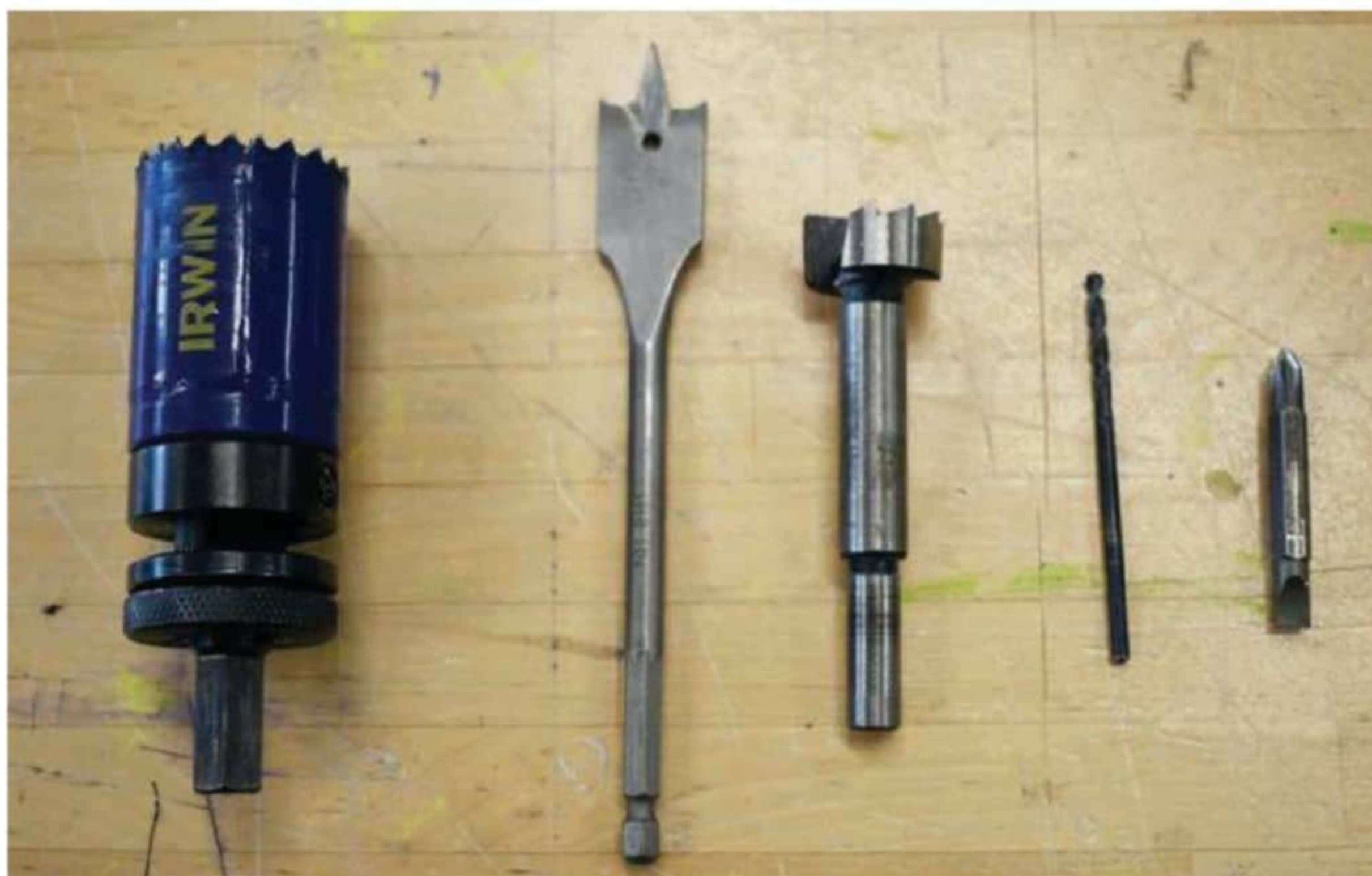
Common bits: Hole saw, Forstner, spade bit, twist drill bits and screwdriver bits
