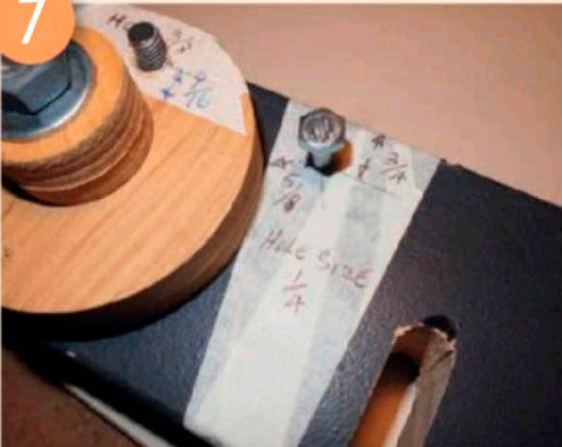
Cut the thread of the 1/4-inch bolt so you end up with a pin about 50mm long
