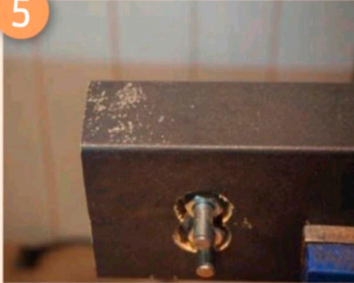
Bolt the two bending pins using the four nuts and washers
