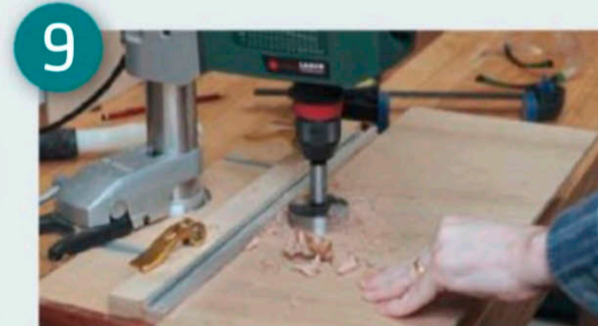
Using some scrap plywood or MDF, 6mm or thicker, drill a hole through the template
