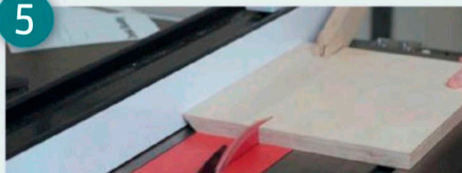
The rest of the cabinets parts can be safely cut at the table saw
