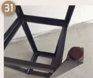
Felt stick-on leg tips were added to the tabs on the bottoms of the legs
