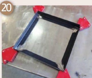
Magnets were used to hold the pieces in a perfect square
