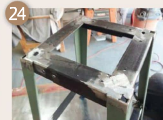
At this point, all accessible welds were cleaned up with a 40-grit flap disk on an angle grinder
