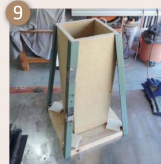
The beauty of using this form is that it helps you precisely mark the legs
