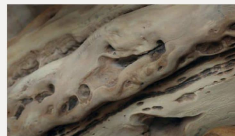
There are a number of insects that eat wood; the damage they cause ranges from minor to catastrophic
