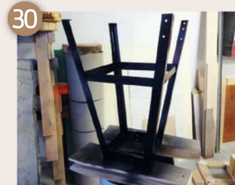
The stool frame was spray painted first with a coat of primer
