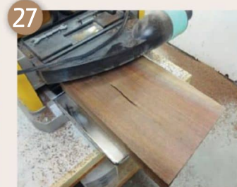
These boards were cleaned up further by running them through a planer
