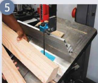
5 The front section of the chair will be cut at an angle to match the sides
