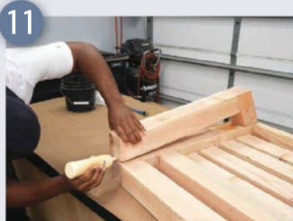
11 When gluing, focus on one section at a time
