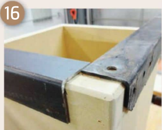
The top of the stool was made with four pieces of angle iron
