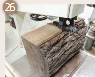
I cut it into two 58mm thick boards
