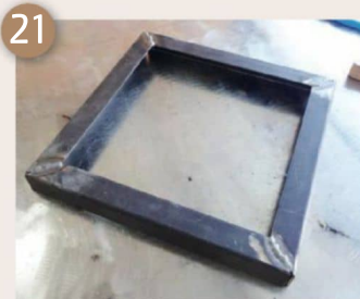
These were tack-welded first, and then got a full bead welded at each joint
