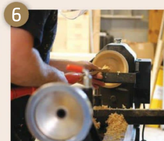
6 With the bowl on the chuck, start to rough out the inside of your bowl
