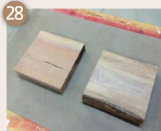
The final seats are 50mm thick and 255mm square
