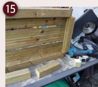
Repeat the process using the 120cm plank with the cut out and a 110cm blank
