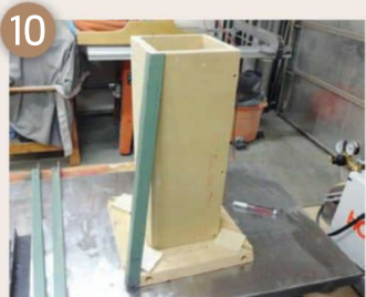
The lower end of each leg was marked and cut first
