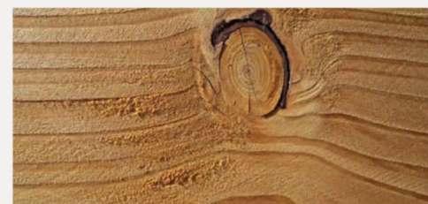
A knot is the base of a branch or limb that was broken or cut off from the tree
