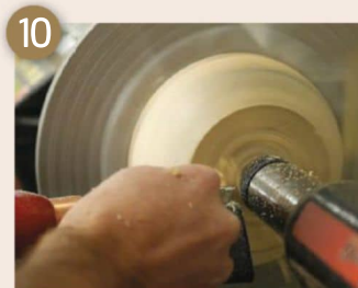
10 Cut away the tenon you created in the previous step
