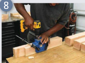
8 Clamp the jig on and line it up
