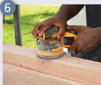
6 I passed over it with an 80 grit sandpaper first, 120 grit
