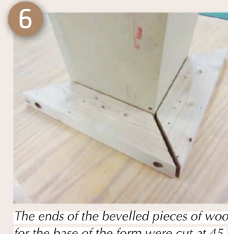
Using a measuring tape and a bevel gauge, I found the required angle
