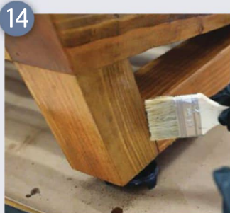
14 And then varnish to seal and protect
