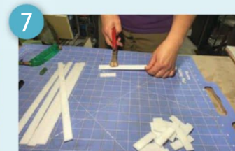
Place the sheet glass on a cutting mat, score the glass with a glass cutter and break the strips apart with the running pliers
