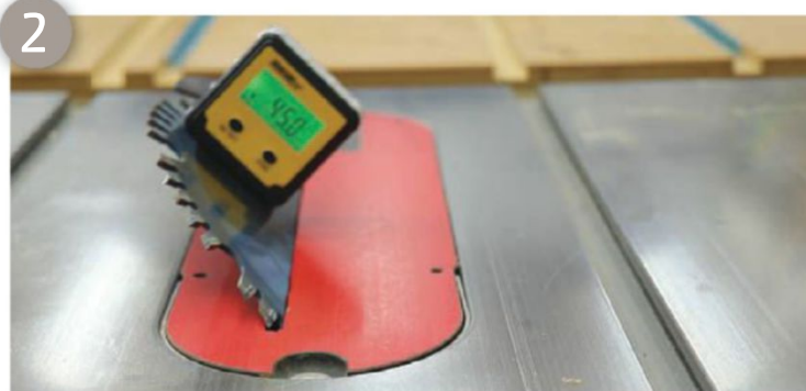
I always like using this digital gauge to make sure my blade is set at exactly 45 degrees.
