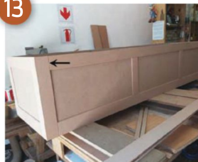
V formed by chamfers
