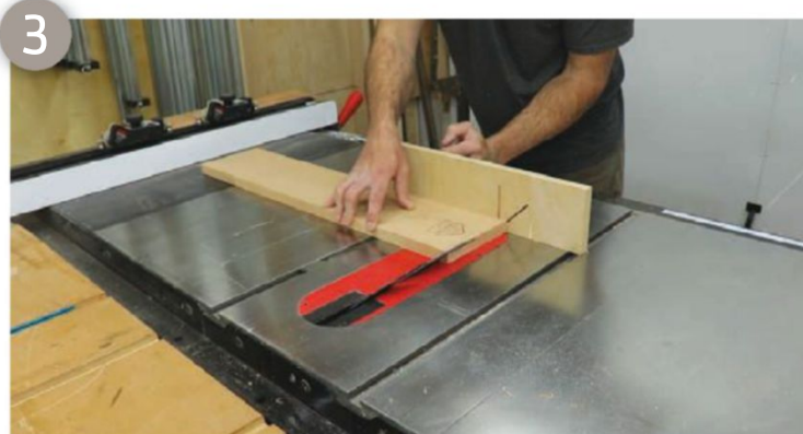
I cut mitres at the very top of each side and on one end of the first shelf
