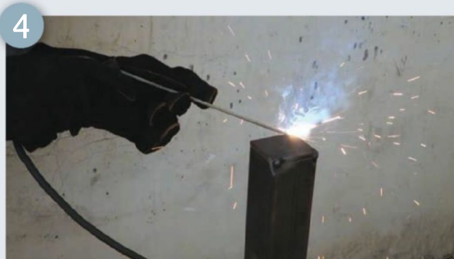
Weld a plate for each leg
