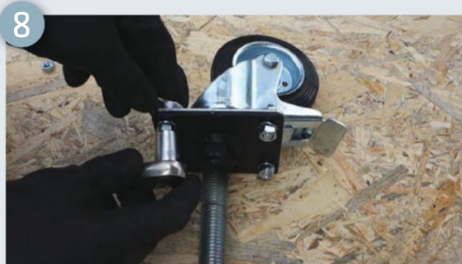
Place the castors on the plate
