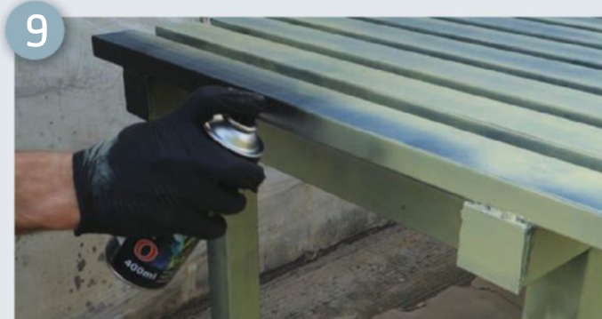
For paint you need to cover the working surface and paint it with primer
