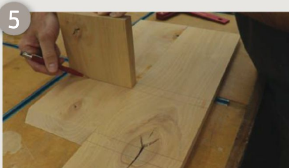
I used the actual shelf to make marks where the dados needed to go
