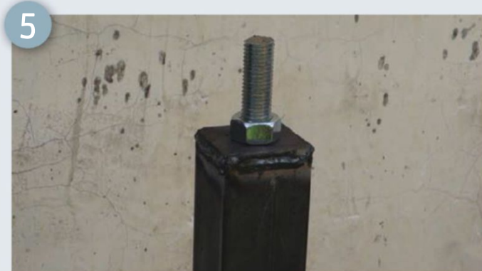
Drill a hole in the centre for a M20 thread rod
