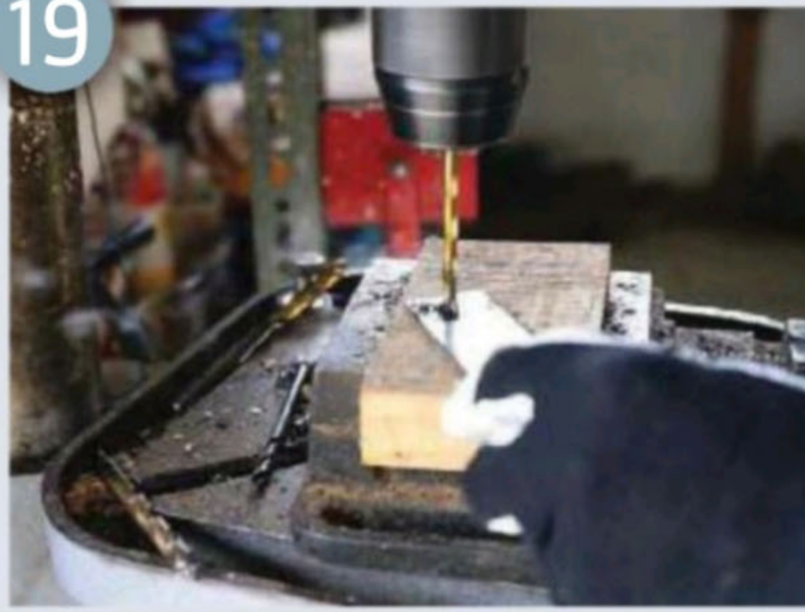
Drilling three holes to provide some adjustment when fixing it to the fork
