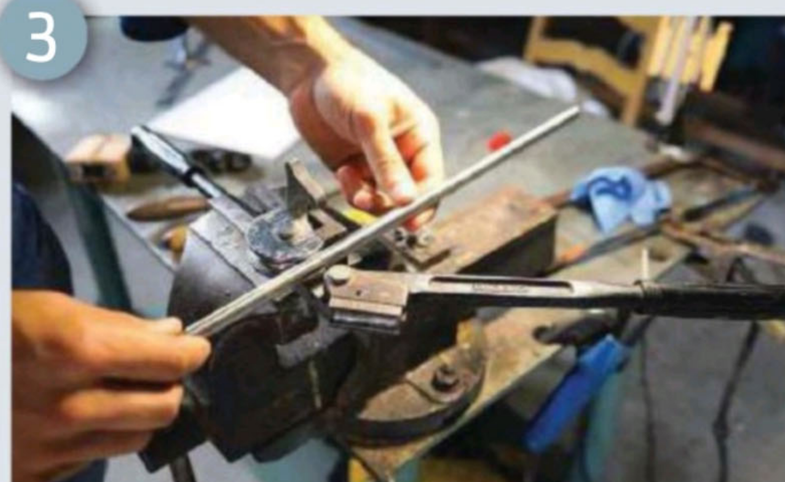
I fixed the bending tool on a vice plane
