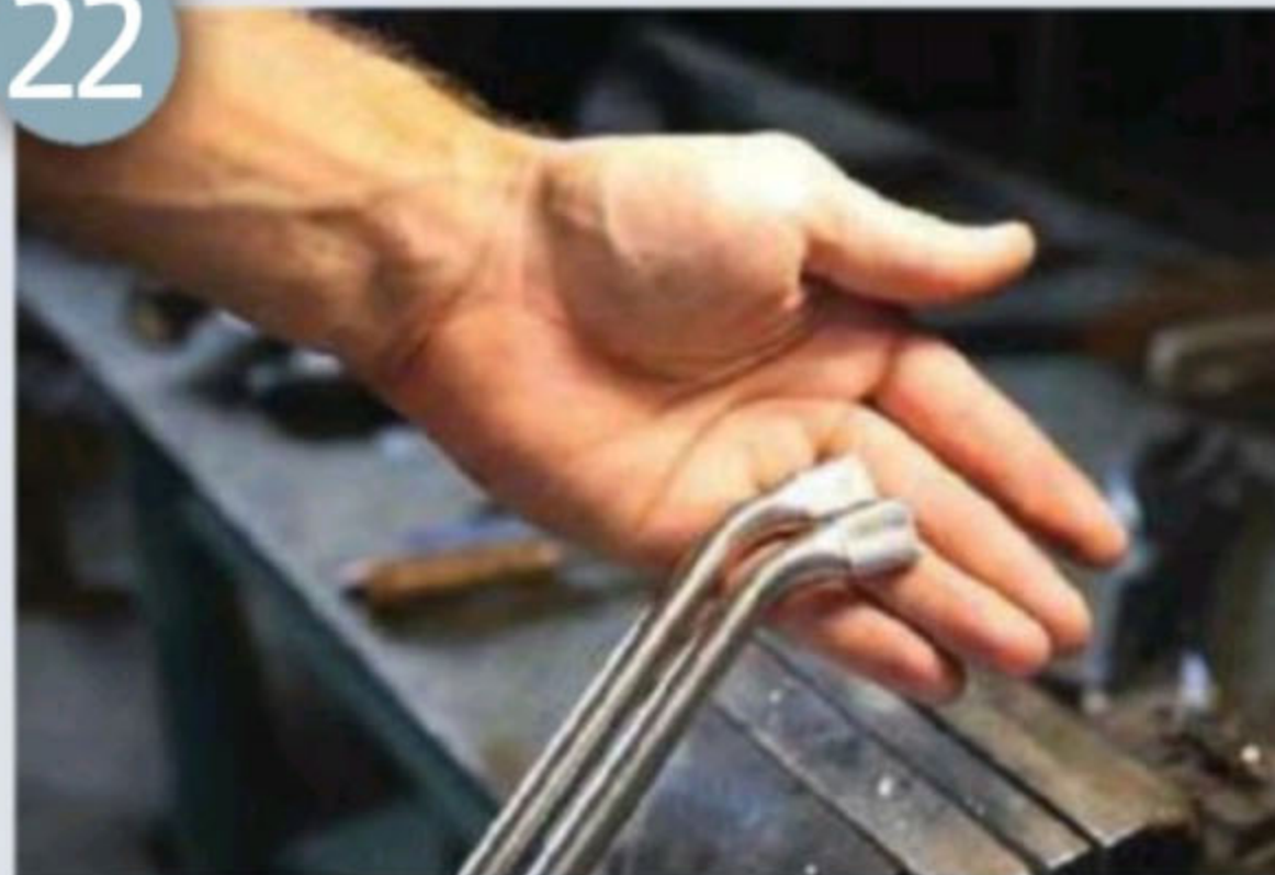
In my case I had to bend the tubes close to these flat surfaces in advance because the tube would touch the fork legs
