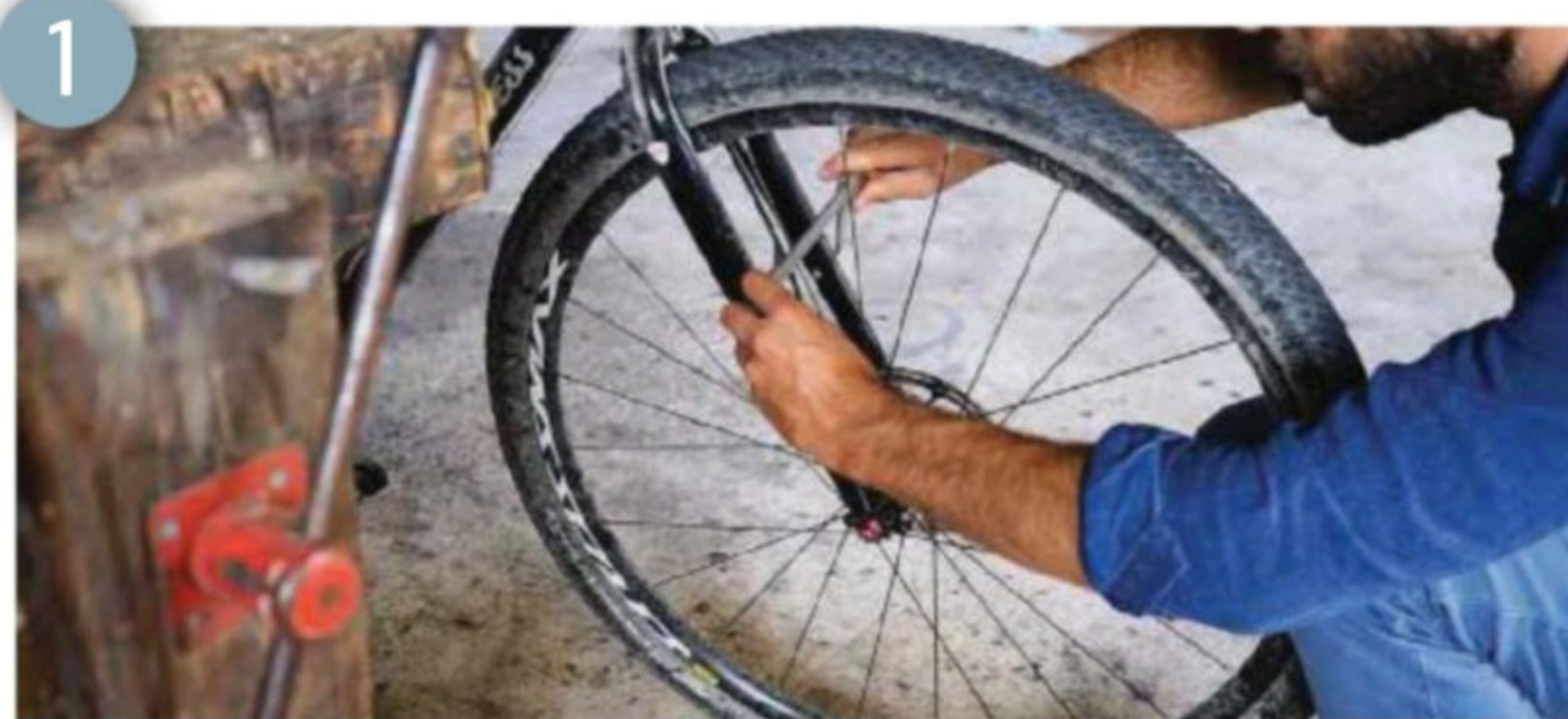
I measured the width of my fork legs at the bolt locations and fixed that as my reference
