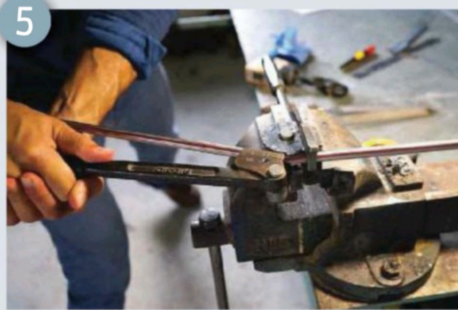
Take your time to bend the tube, particularly stainless has it is quite hard to bend
