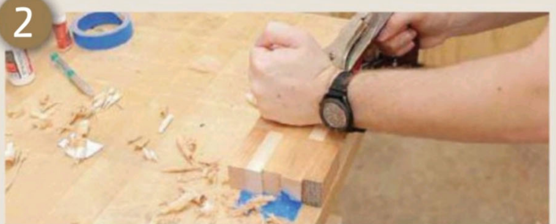
Because the scrap wasn't thick enough, I had to cut it down on the table saw, then used a hand plane to flatten it
