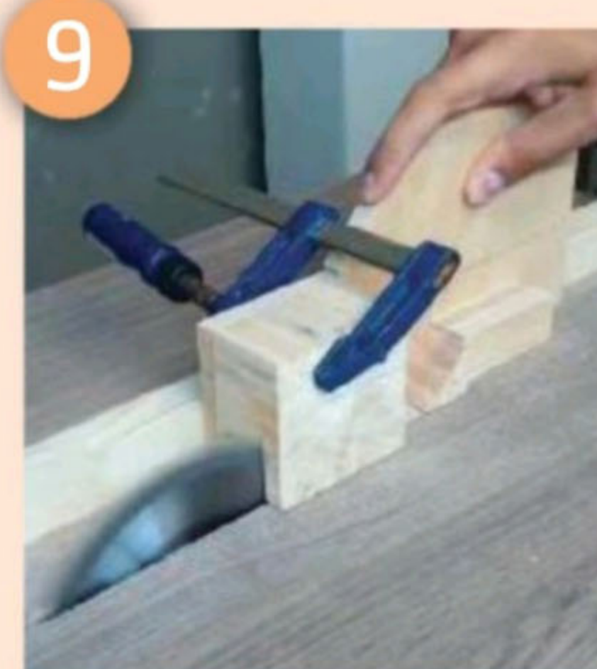
Using the jig to help cut the blocks
