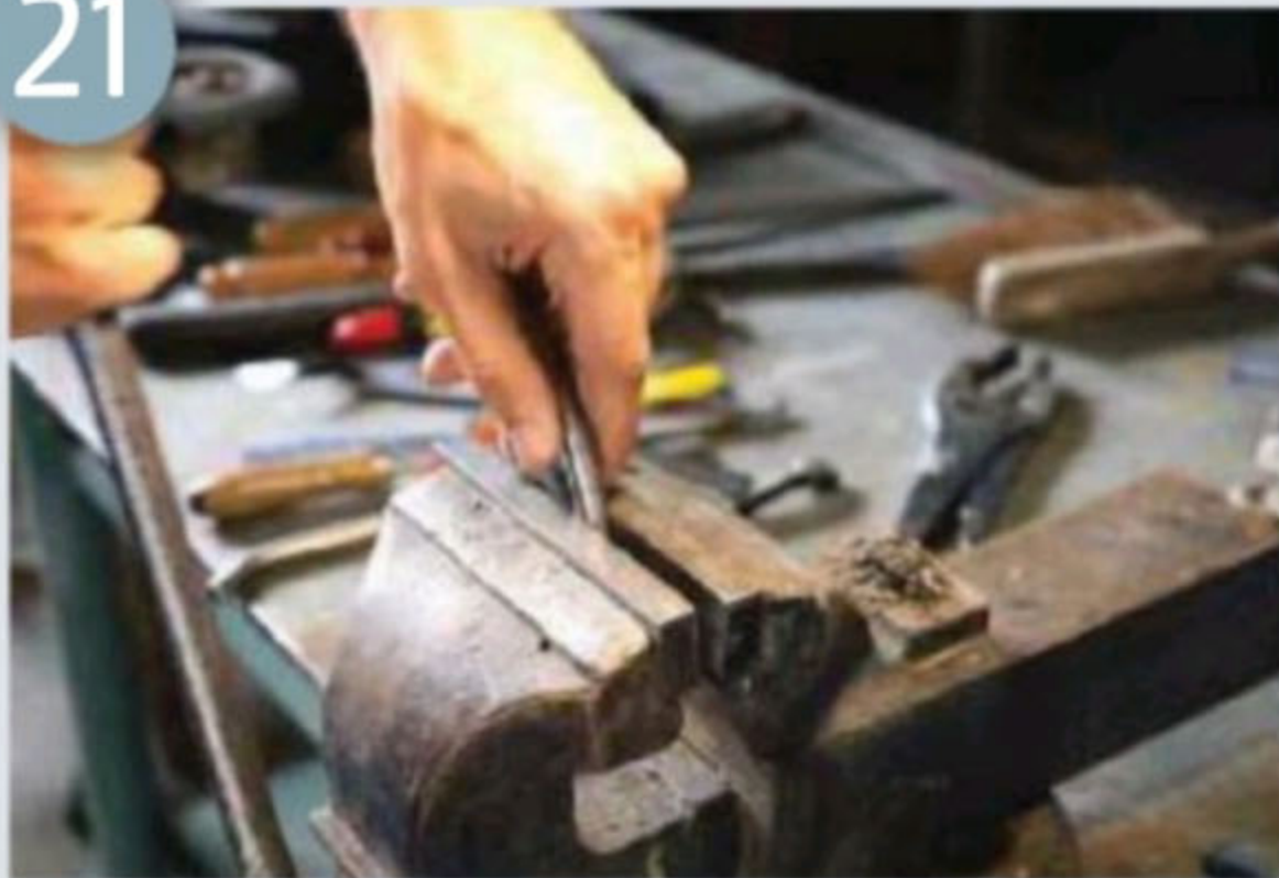
With the vice, I just created a flat surface to provide an attachment point through a bolt by crushing the tubing
