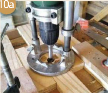
Figs. 10A and 10B: Drill set-up – drilled out waste area
