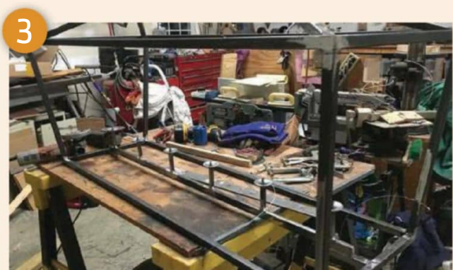
In order to keep the wiring hidden, I welded a 12,5mm square tube to the centre of the lower ends
