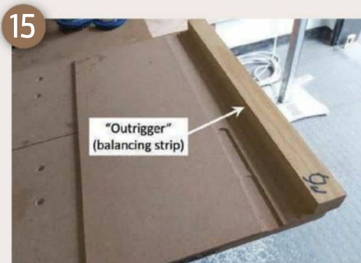
Balance with an 'outrigger'
