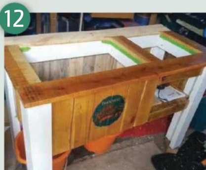
12 Once the pallet wood was all fixed in place I gave it a couple of coats of clear outdoor varnish to give it a nice shine
