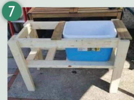
7 Once the top and bottom frames were assembled, I attached the legs
