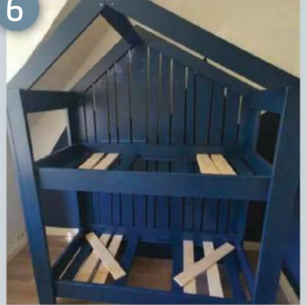
Add a second support beam on the front with an extra plank across the tip of the roof for extra strength
