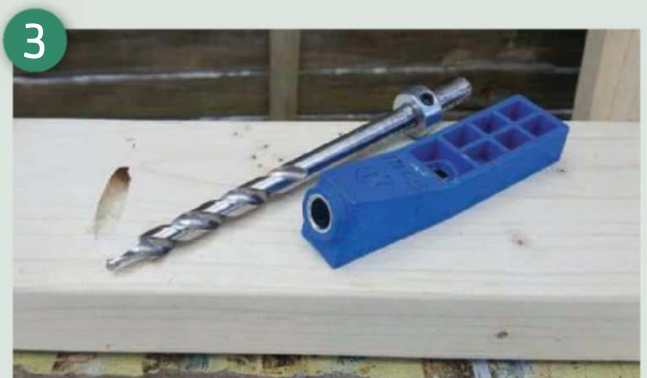
I joined two pieces of 90mm x 38mm timber together with pocket screws
