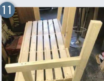
11 The angle of the back support is quite important
