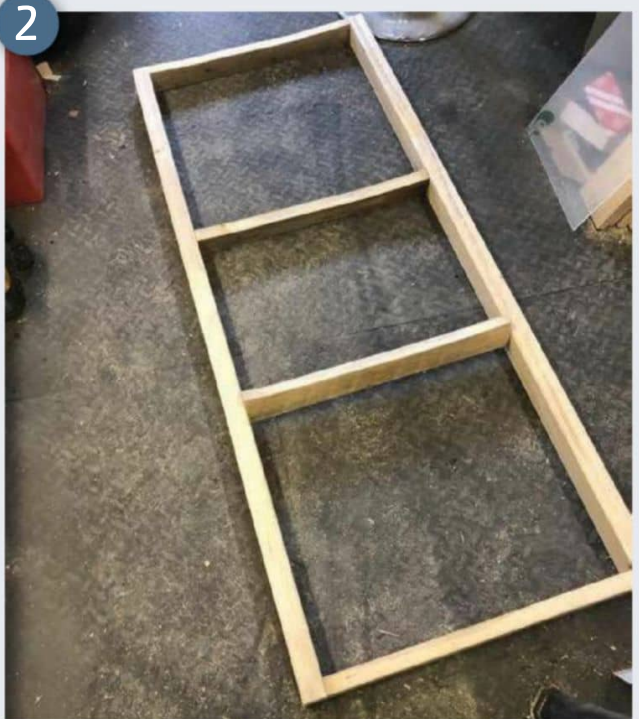
To start I cut to length the radiused supports at 500mm
