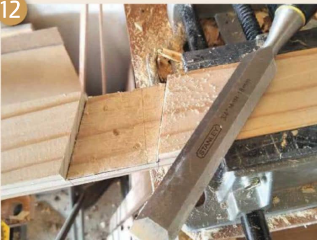
Fig. 12: Cleaning-up joint with a chisel
