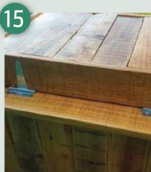
15 I then screwed the frame to the lid itself and giving it a couple of coats of varnish
