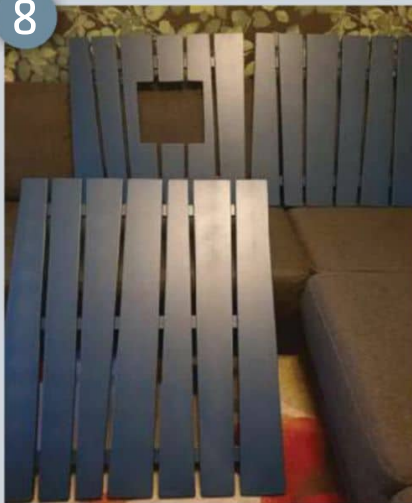
On the inside of the doors we made used strips to hold all the planks together
