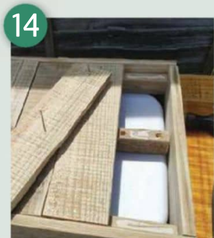
14 After putting the cool box in its place I put the lid on and built a wooden frame around it
