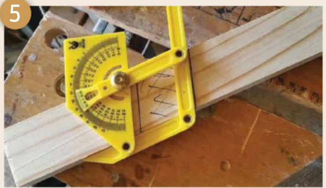
Fig. 5: Marking the section on the workpiece. The width of the material is then marked, and the second cut line marked. The area to become the lap-joint is shaded
