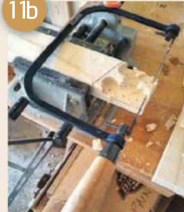
Figs. 11A and 11B: Using a hacksaw and using a coping saw
