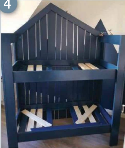
The back panel in place
