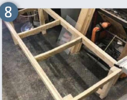
8 The slats ready to be installed
