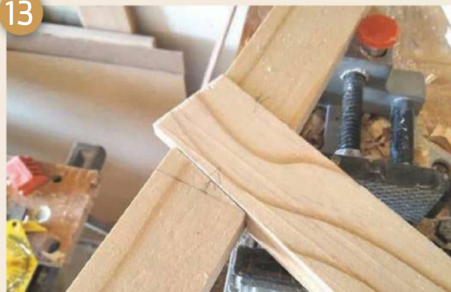
Fig. 13: Test fitting joint
