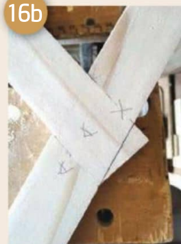
Fig. 16A and 16B: Mark-off ends and score across grain. Cut and trim
