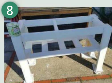
8 Next give the whole frame a quick sanding and a few coats of outdoor paint
