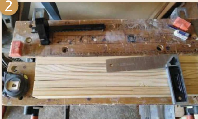
Fig. 2: Check ends square and all pieces are the same length
