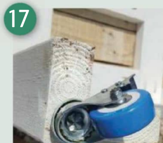
17 To fix these in place I drilled a hole in the bottom of each leg and used some threaded inserts to enable me to adjust the height of each wheel
