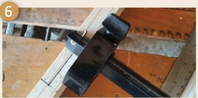
Fig. 6: Using a marking gauge to score a line half the thickness of the timber
