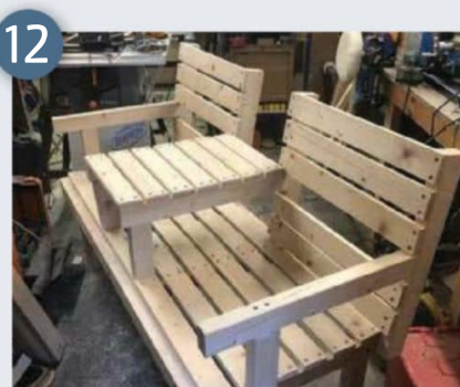
12 The back supports and arm rests installed
