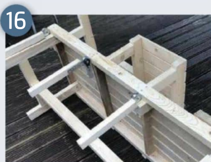
16 Next job was to make some side pieces for the footrests
