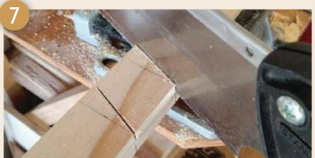
Fig. 7: Sawing to the inside of the marked line down to half the thickness
