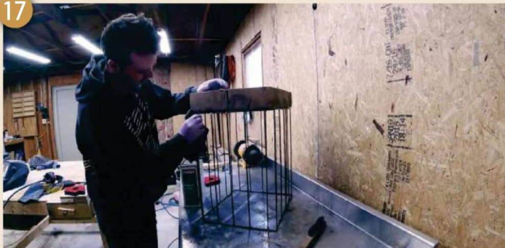
Clean off the steel with a steel brush and mineral spirits
