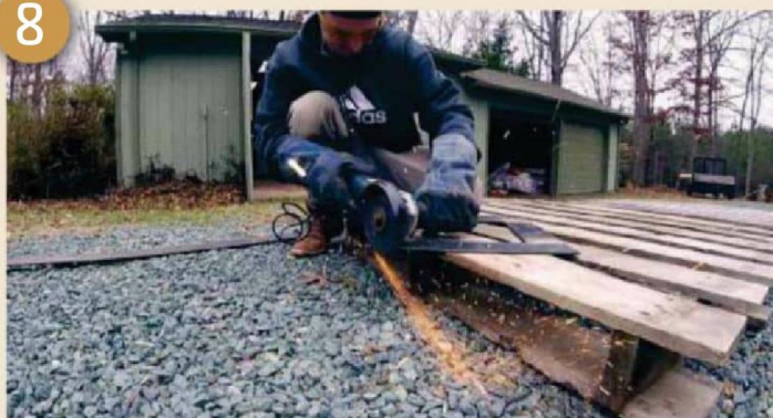
Trim off the corners of the bracket
