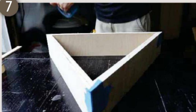
Using painter's tape while the glue sets before nailing
