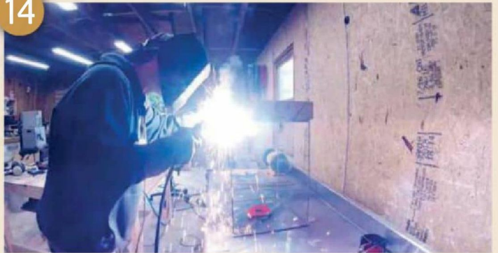
Weld five pieces of the 500mm lengths of steel rod to each side of the table
