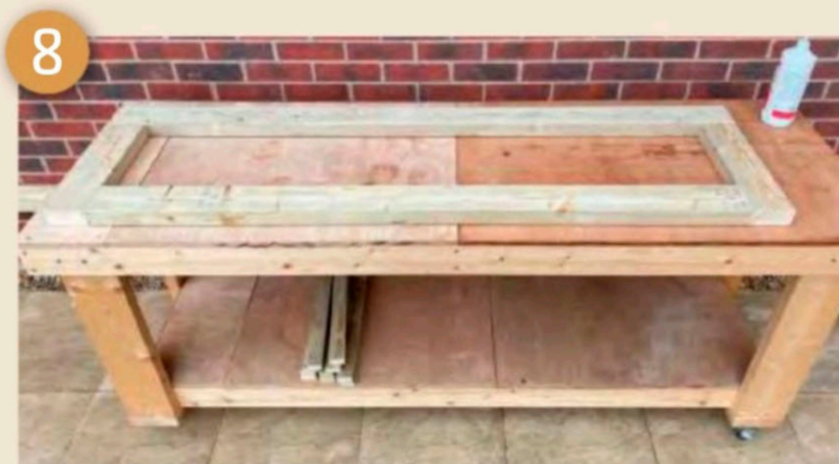
To keep things square, cut another piece of wood to stop the legs bending in or out during clamping
