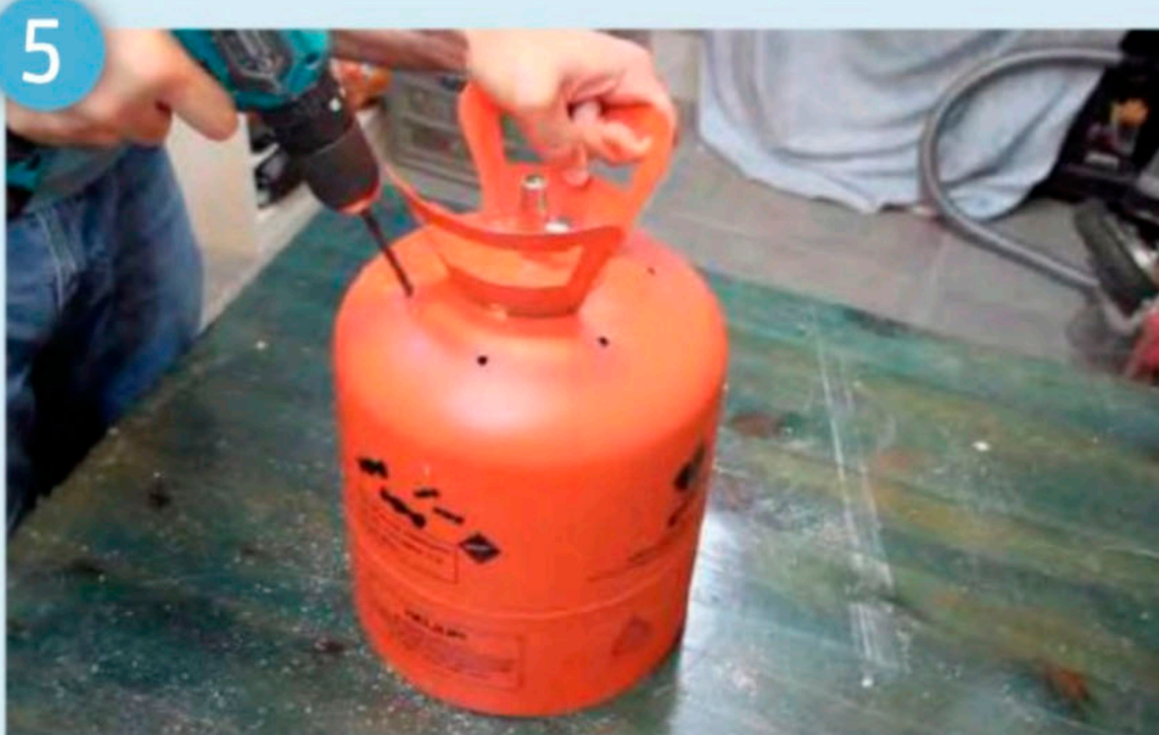
5 Drill drainage holes
