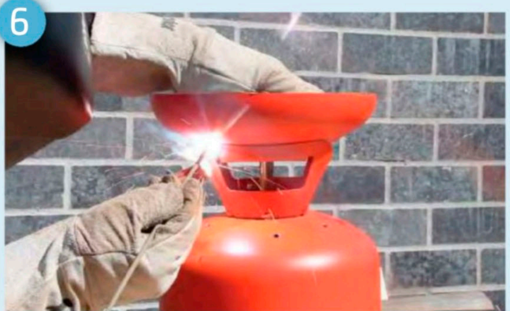
6 Welding the off-cut onto the valve guard
