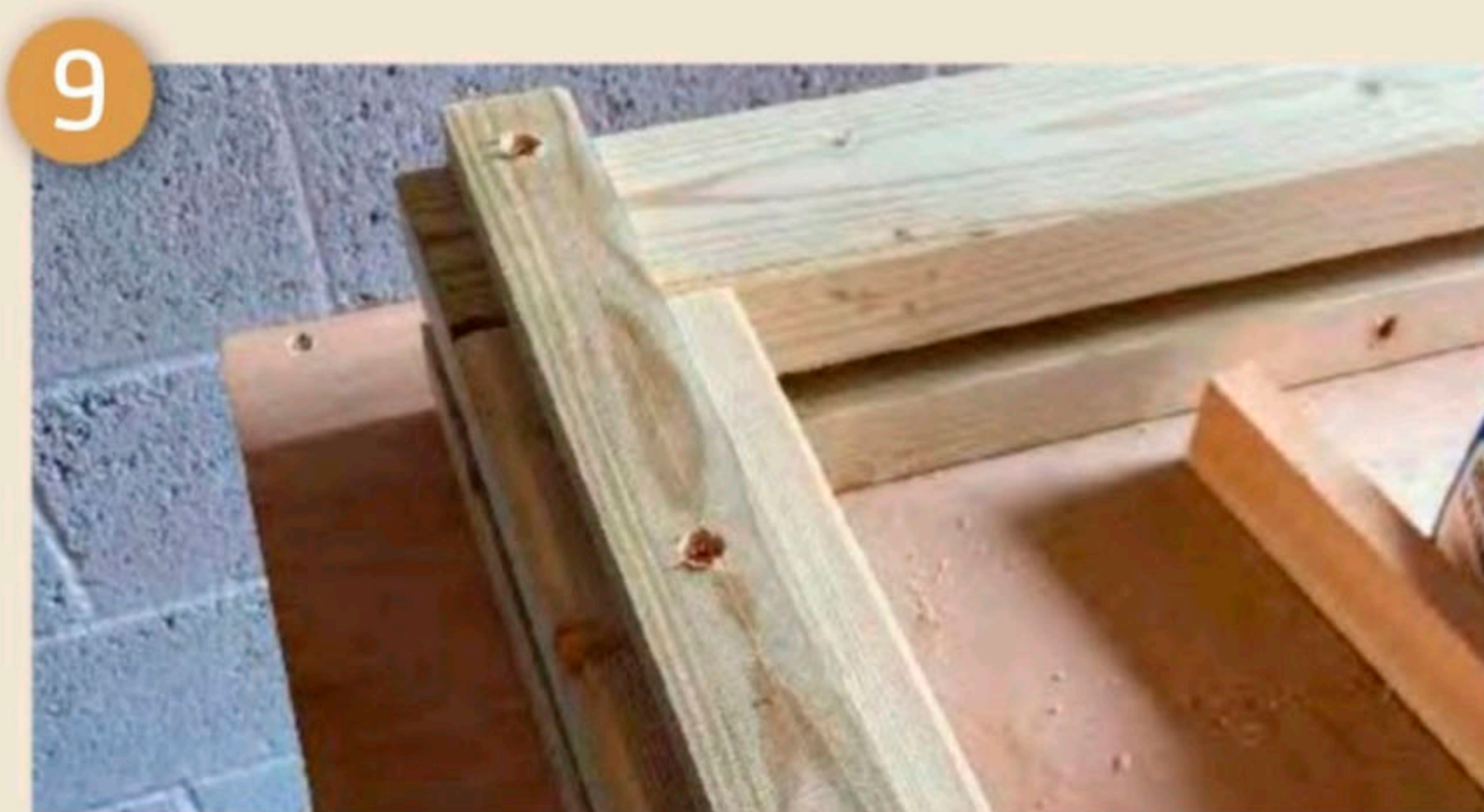
You should now have six beams each with a pair of legs that are ready to be joined together using the smaller piece of wood
