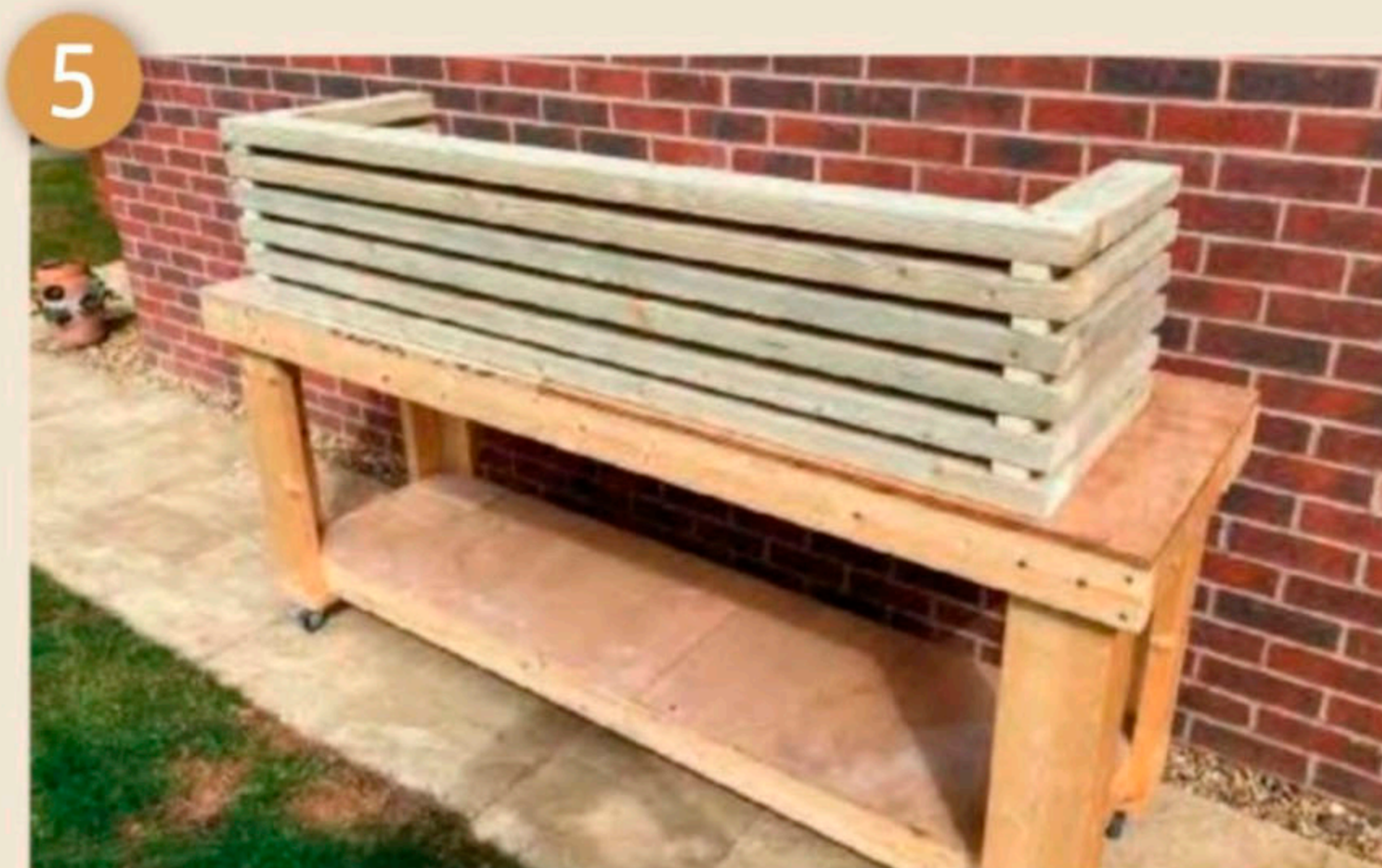
Dry fit the pieces together
