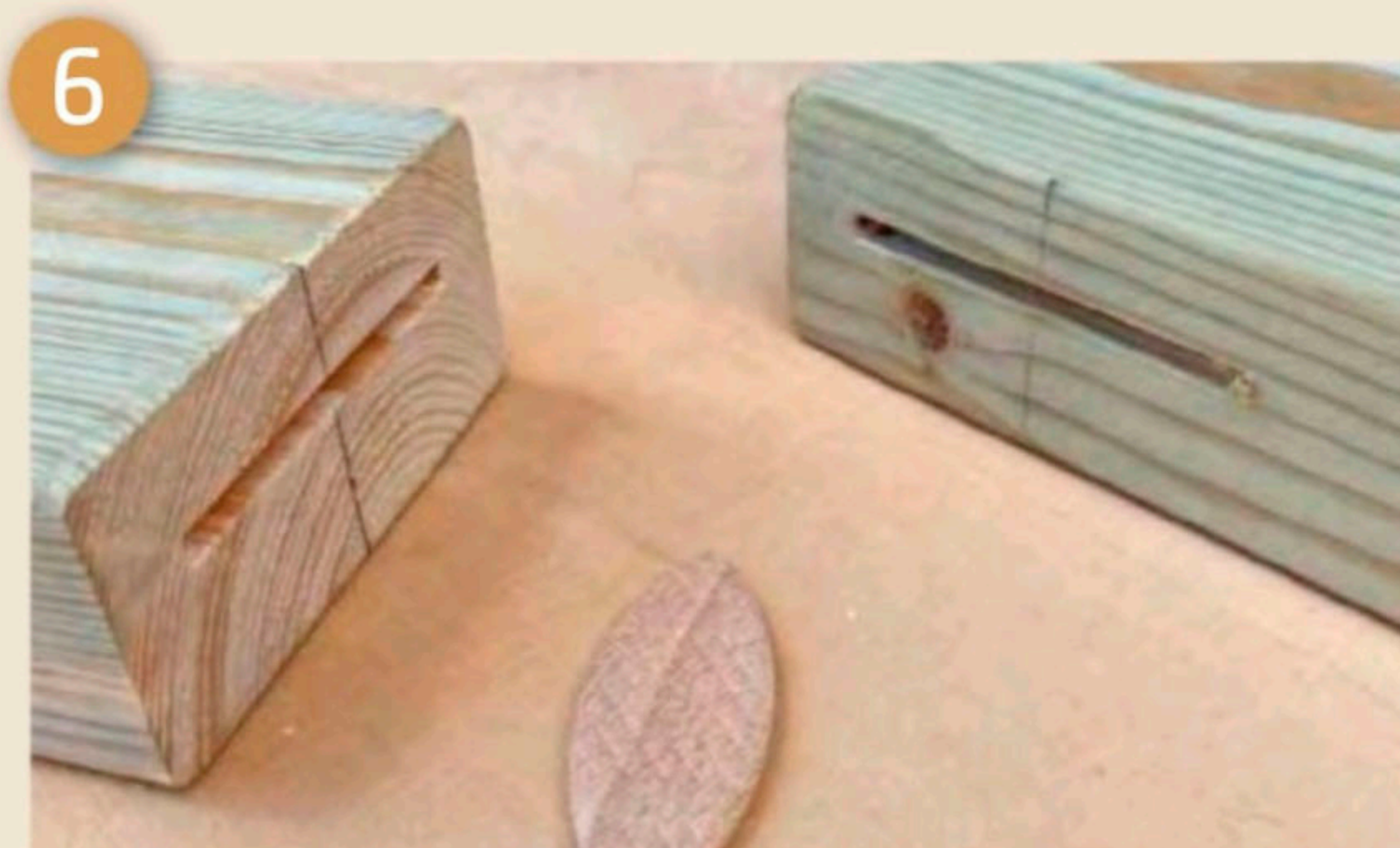
Biscuits and glue were used to attach the legs and beams
