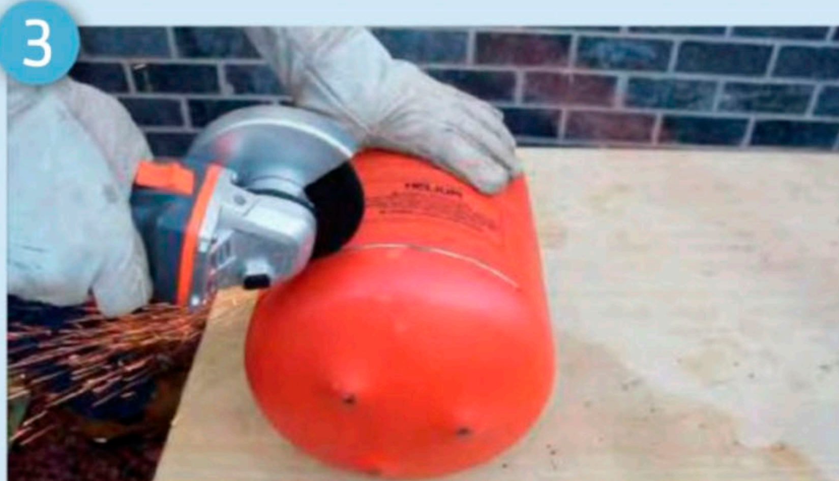
Cut the cylinder with an angle grinder
