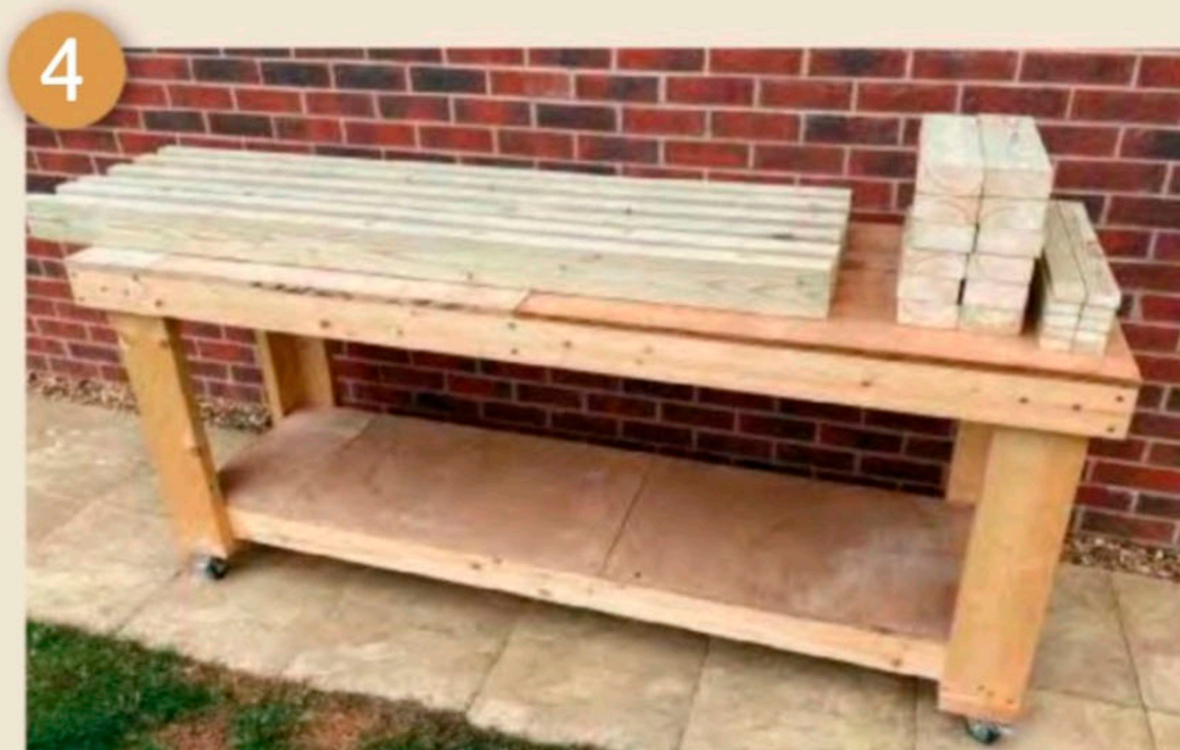
Once it is cut to size, sand everything with P80 grit
