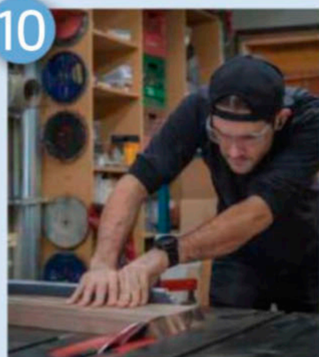
Cutting the wood at 30°
