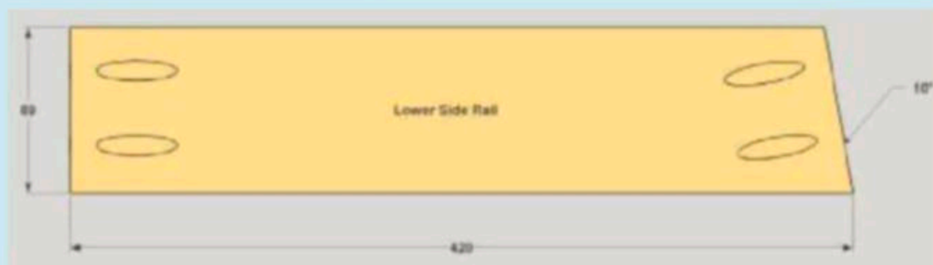
Cut a pair of Lower Rails
