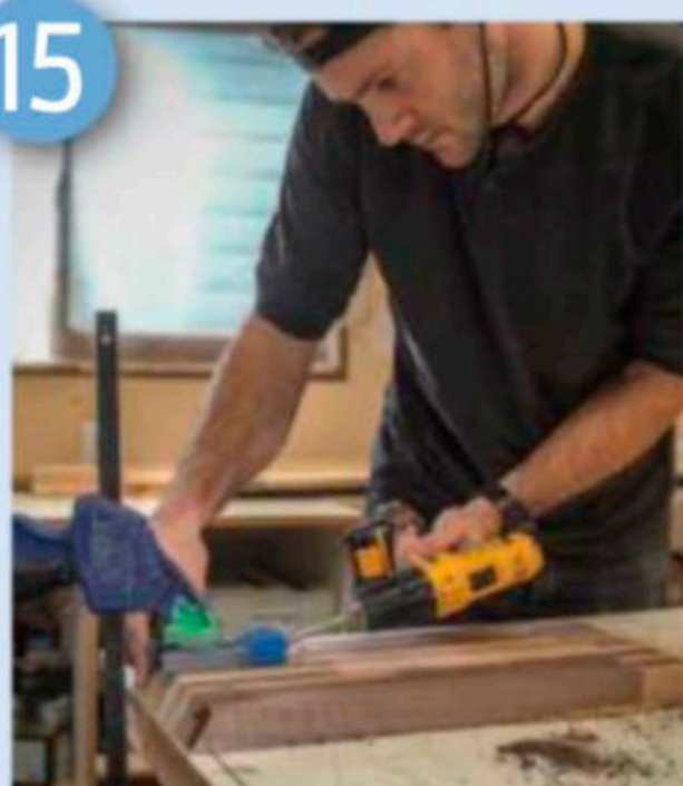
Pocket screws were used to secure this project
