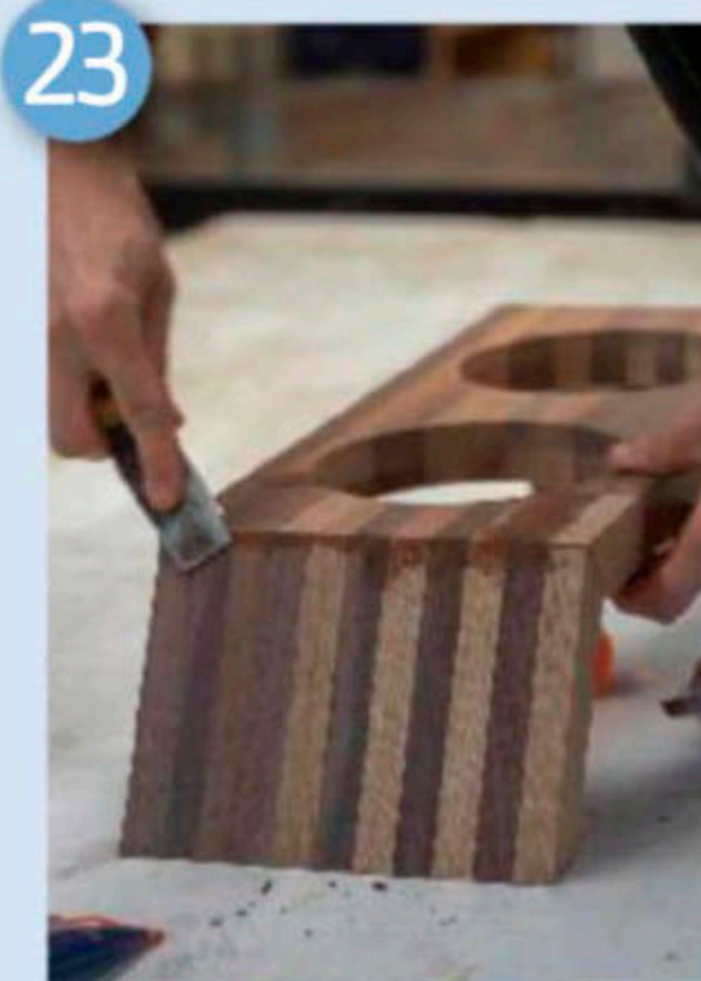
Any small gaps and imperfections were filled with wood filler
