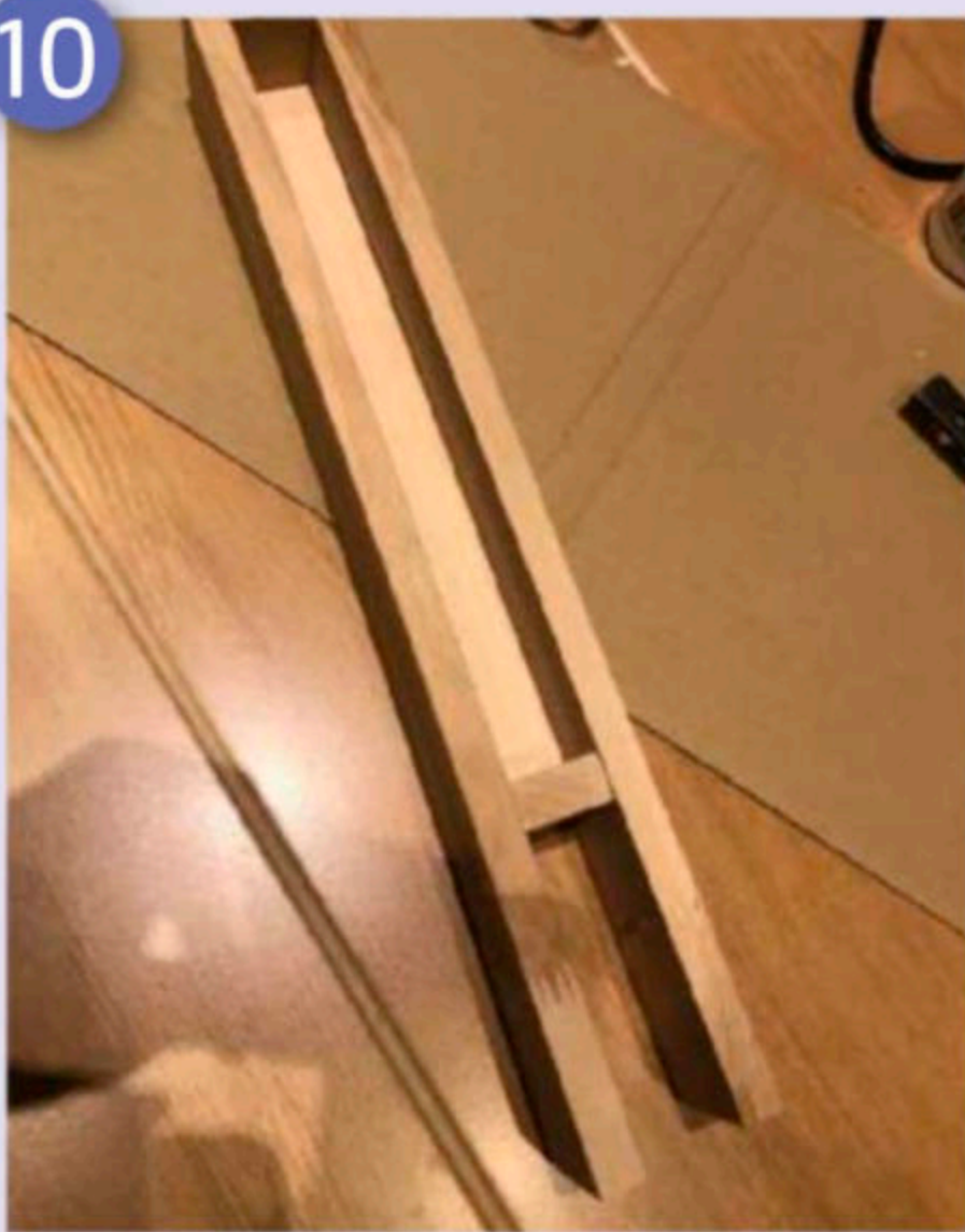
Take remaining pieces of wood and glue with wood glue
