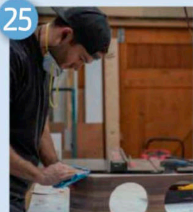
After sanding, and before applying the finish, give it a good wipe down
