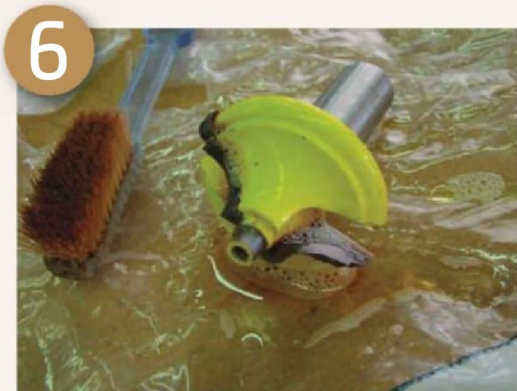
Cleaning a bit
