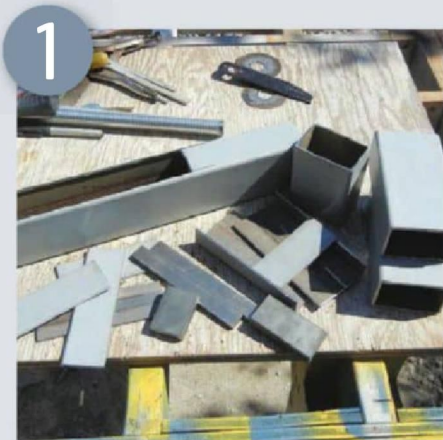
1 I used rectangular tubing for the majority of the vice. Here are all of the parts cut and ready to assemble
