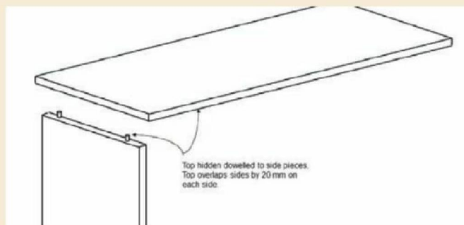
Fig. 5: Dowelling the top
