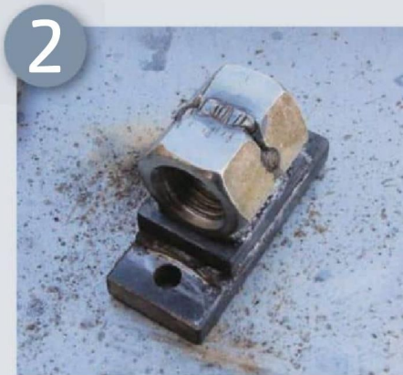
2 The vice uses a 1-inch threaded rod as a lead screw and what it screws into must be strong. I've used two nuts, welded to two thicknesses of steel bar stock
