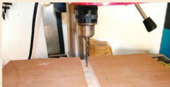
Fig. 3: Preparing the dowel fixing to the sides
