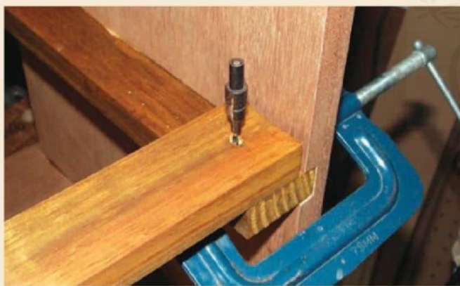
Fig. 8: Clamping the side supports in position; positioning and marking the cross stretchers
