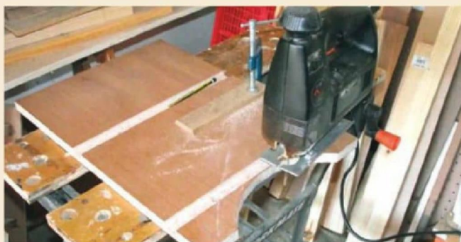
Fig. 6: Cutting the curve on the side supports
