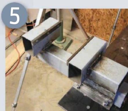
5 This vice has a fairly large capacity, with 150mm wide jaws and more than 150mm throat depth
