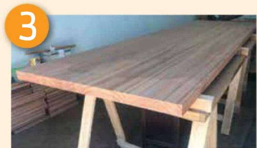
The four pieces of kiaat glued together to make this 3100 mm x 900 mm tabletop were edge trimmed, prior to gluing, with a hand-held router and straight edge
