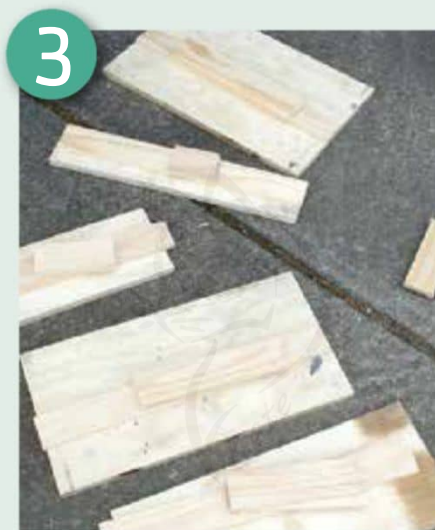
Cut your plywood to size which will be used for the wooden shelves
