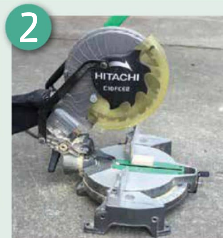
A mitre saw was the main power tool used for this project
