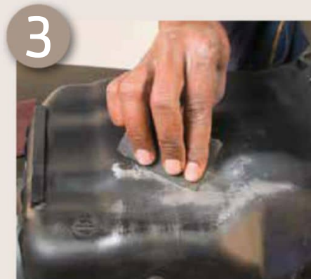
Sand the area around the crack
