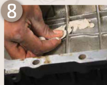
Knead and wipe the putty onto the surface around and over the crack
