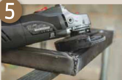
Go over your welds with an angle grinder
