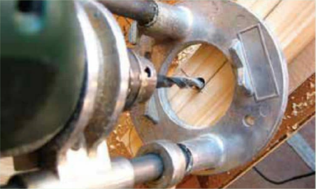
Fig. 4: Drilling the jigsaw pilot holes
