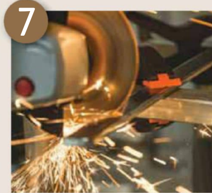
Cut some tabs to hold the wood and foam base onto the frame
