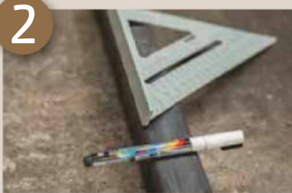
Make a series of mitre cuts at 45°
