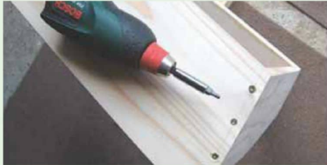
Fig. 13: A completed side and end piece joined
