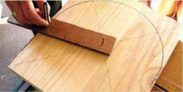
Fig. 3: Marking the wheel diameter
