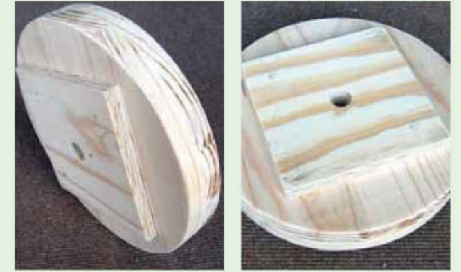
Fig. 11: The completed wheel assembly The 6 mm hole has been drilled out to 19 mm
