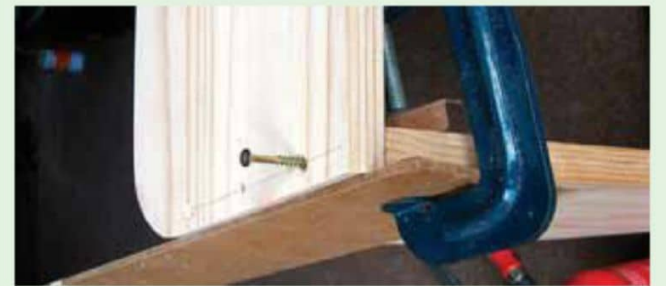
Fig. 12: Lining-up a side piece with an end piece
