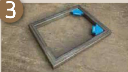
I used some welder's magnets to hold the frame together
