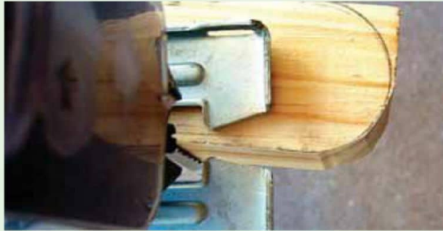
Fig. 6: Cutting the ends of the handle section
