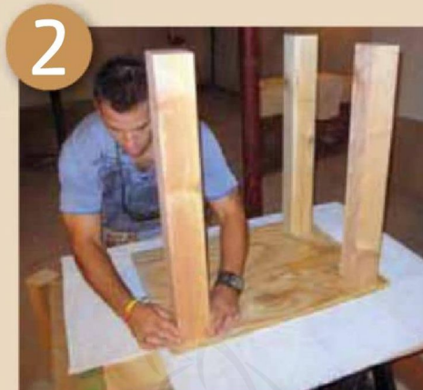
Position the legs on the plywood
