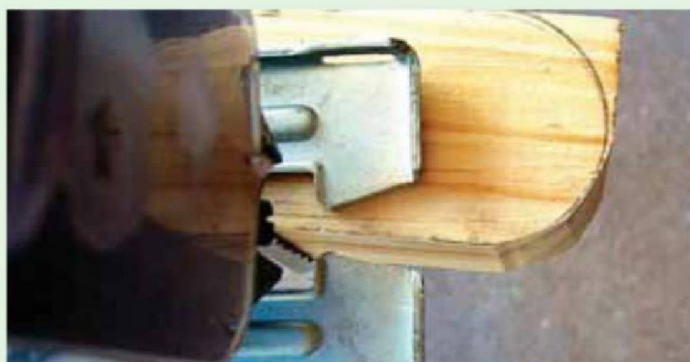
Fig. 6: Cutting the ends of the handle section
