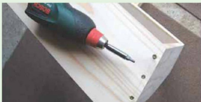
Fig. 13: A completed side and end piece joined
