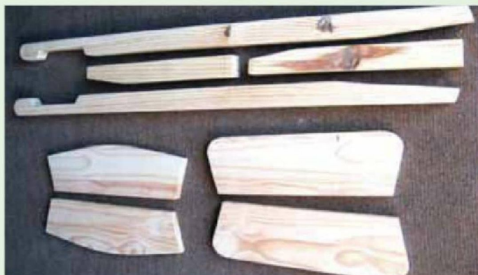
Fig. 10: The shaped and sanded tray, arms and legs
