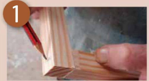
The horizontal must overlap the vertical. Mark the location of the drill-hole
