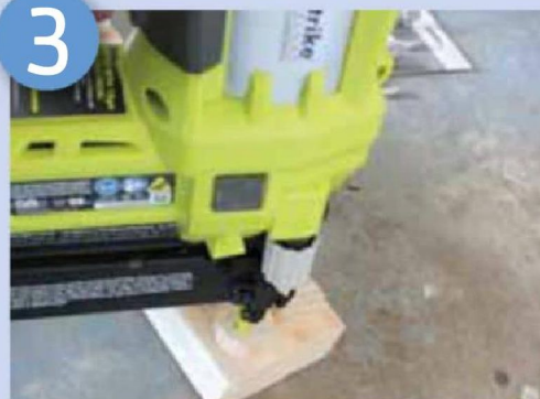
Using a brad nailer to fit the dowels
