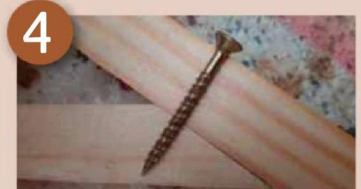
Identify the location of the screws for fixing the diagonal in place, by placing the screw in the ideal position and draw a drill guideline
