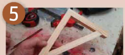
The first bracket will serve as a template for the remainder that you may need, based on the load bearing requirements
