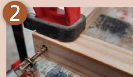
Clamp the loose components in place and fix the joint with cold wood glue and the screw
