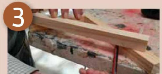
To determine angle to cut for the diagonal, place the timber across the horizontal and vertical portions and mark the underside, where it meets. That will be your cutting line
