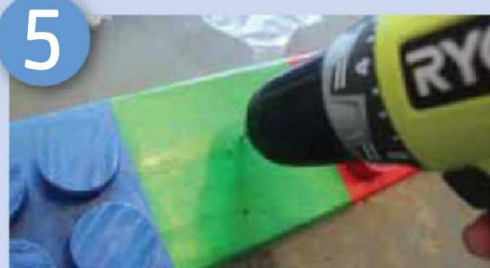
Drilling pilot holes for the hooks
