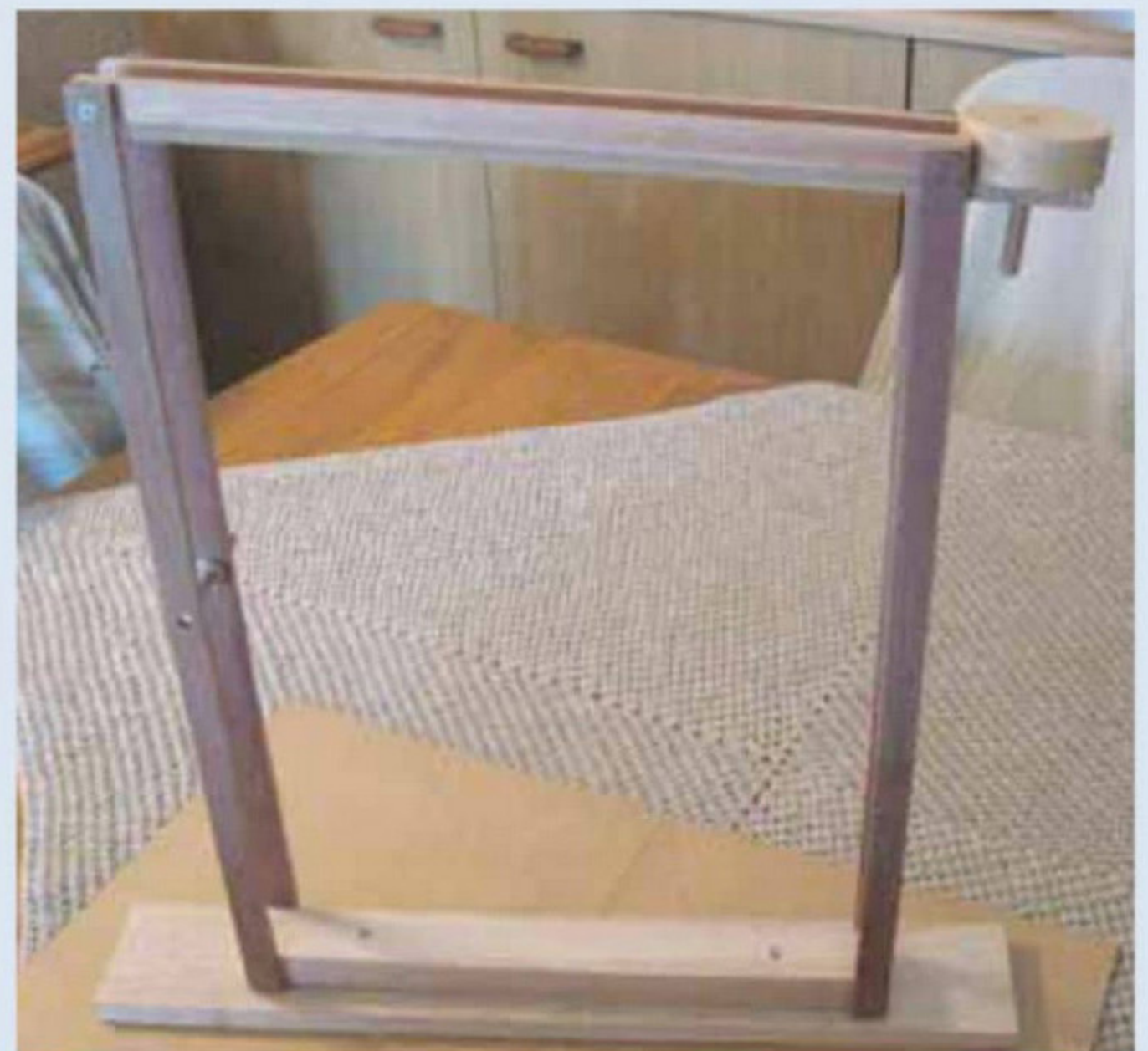
Fig. 3: Finished frame view of the completed frame assembly. The larger base piece had not yet been screwed to the base of the frame assembly
