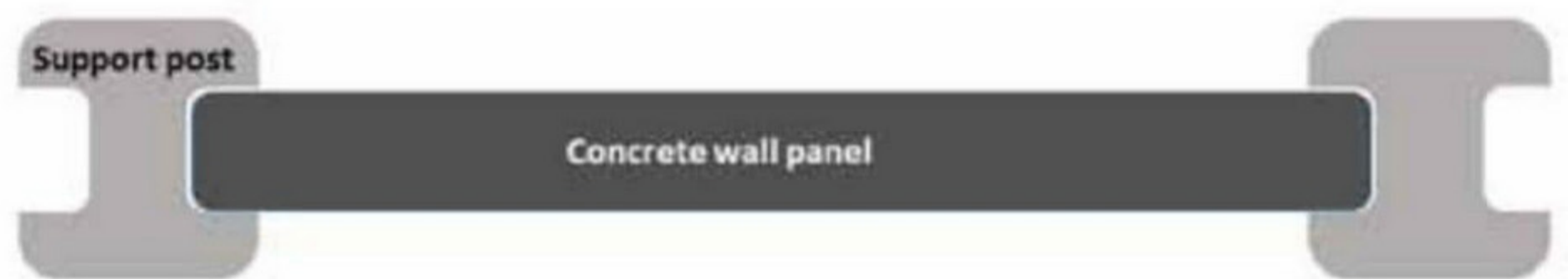
Top aspect of precast wall showing the recess cavity into which the panels slide
